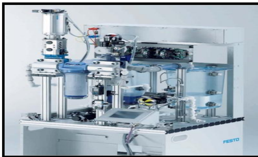
Figure 3.2 : station de filtration
