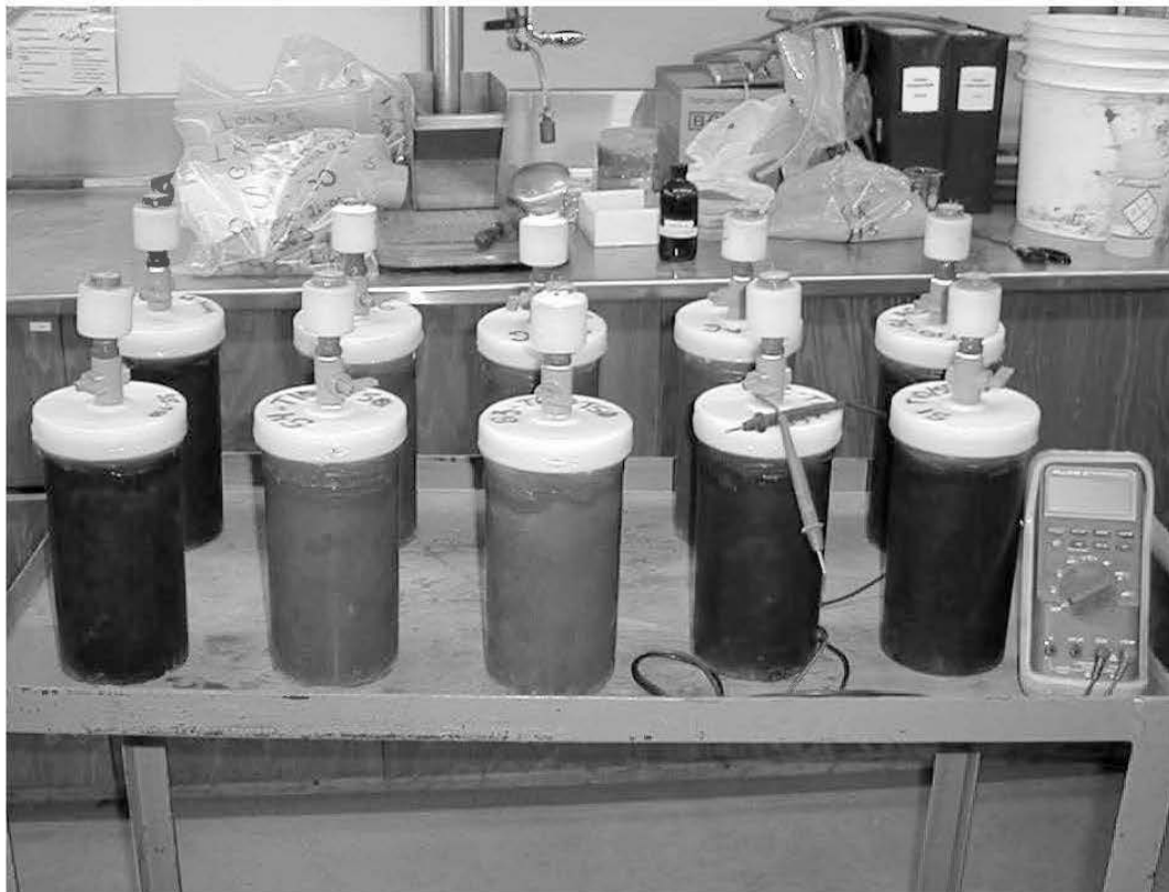
Figure C.2, Oxygen-consumption setup for the CPB samples.
