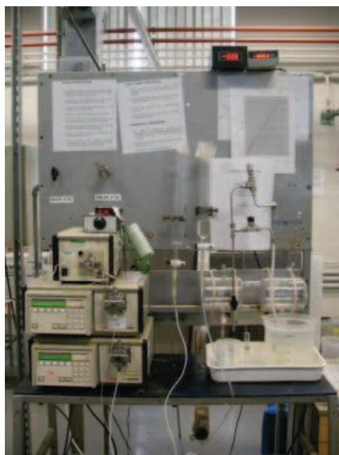
Figure 8.4 Picture of two HPLC pump, a static mixer and feeding columns
