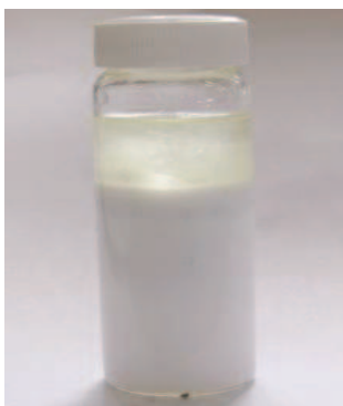
Figure 8.6 Sample of hydrolysed sunflower oil: upper layer (FFA, TAG, DAG, MAG) and lower layer (glycerol, water)
