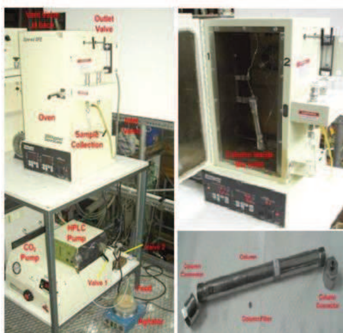
Figure 8.1 Laboratory experimental set-up of continuous extractor equipment (CEE)
