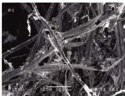
**Figure 3-2 Pâte NBSK R<sub>1</sub> raffinée 15 min – CSF 620 mL**
