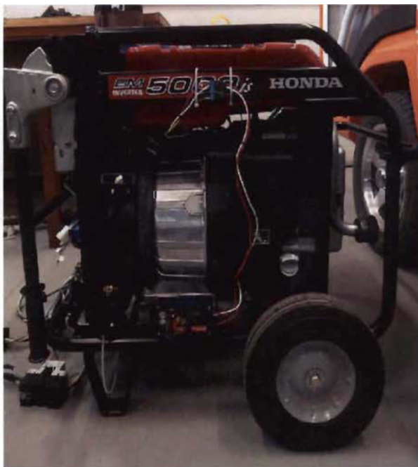
Fig. 5 – Retrofitted hydrogen-based genset.
