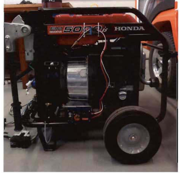
Fig. 1. Genset Equipped with Two Alternators
