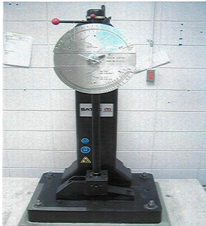
**Figure 3.6** A computer-aided instrumented SATEC SI-1 Universal Impact Testing Machine, with a Dynatup IPM/PC impact testing system for data acquisition.
