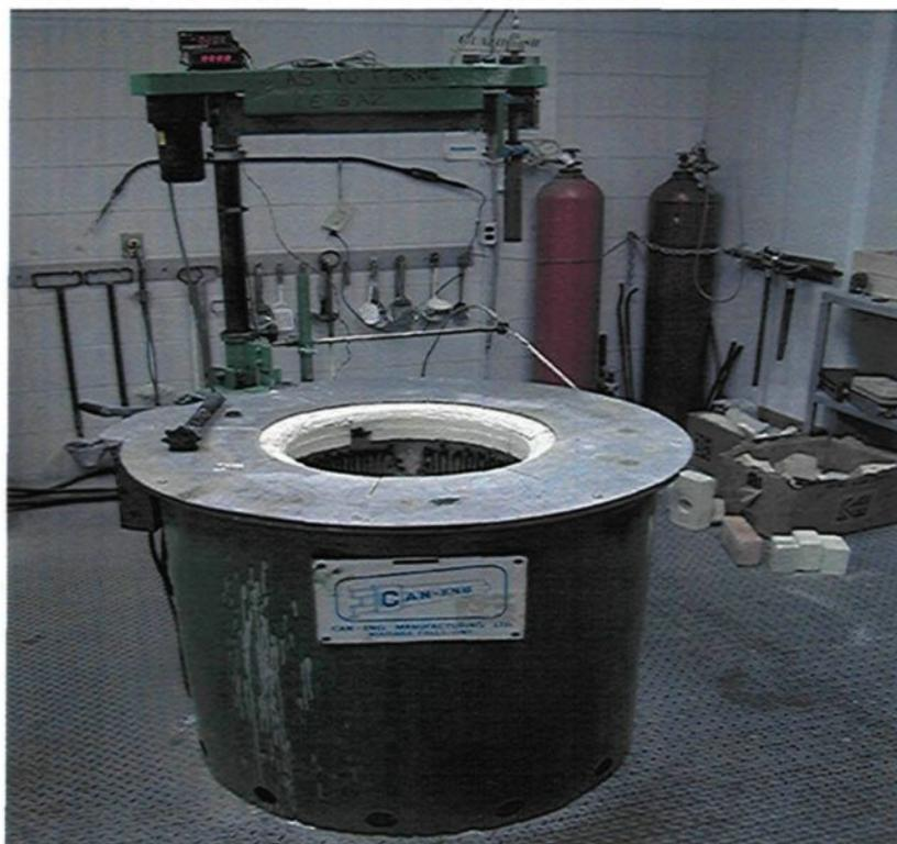
**Figure 3.1** Furnace used for preparing experimental alloys.
