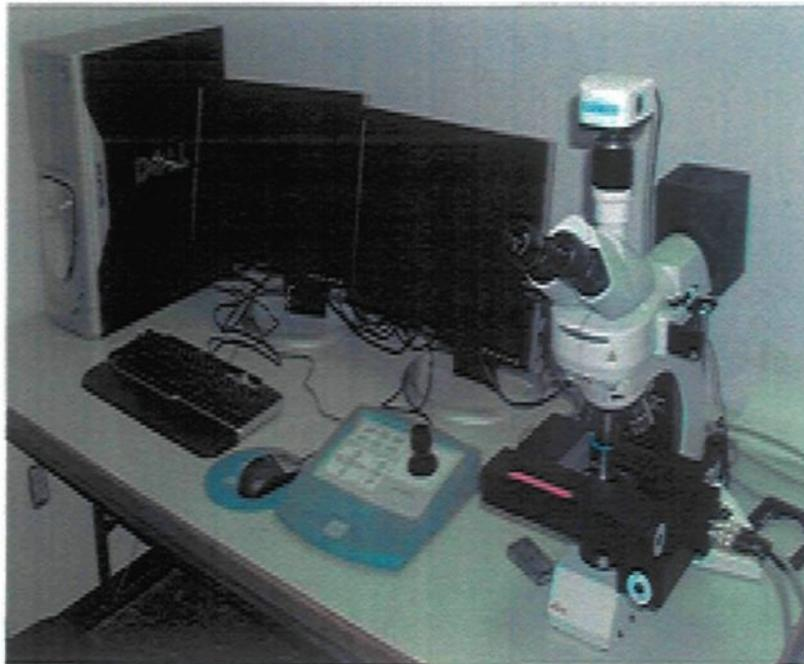
**Figure 3.7** Optical Microscope - Clemex Image Analyzer system.
