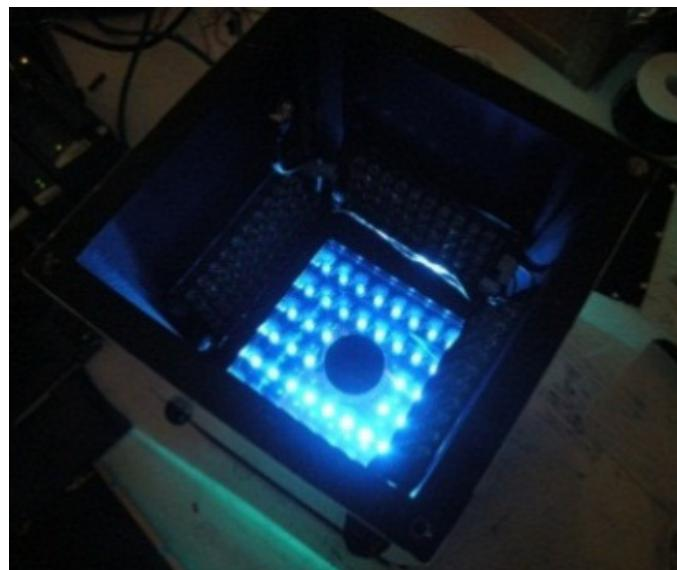
Figure 1.8 TIS-III excitation LEDs behind a band-pass filter
