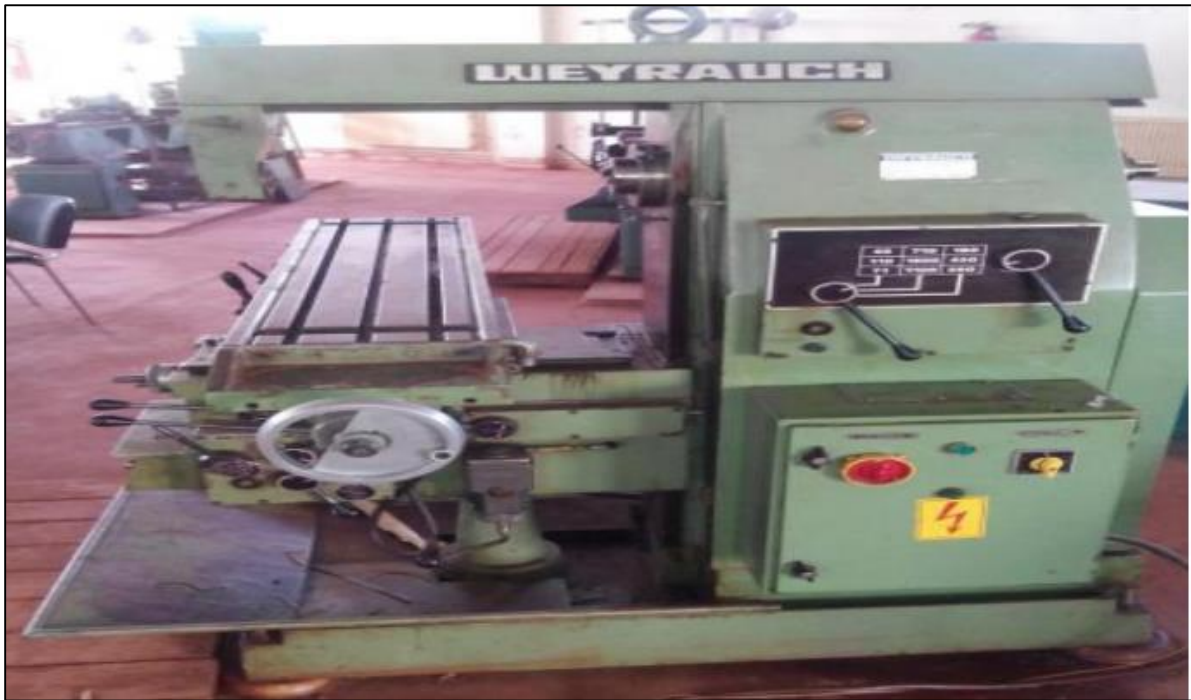
Figure 2.6: Fraiseuse universelle WEYRAUCH FR -U-1100 [13].
