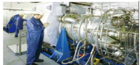
SGT-400 core engine test facility.
