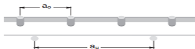
Figure II.6 : L'écartement des stations supports
