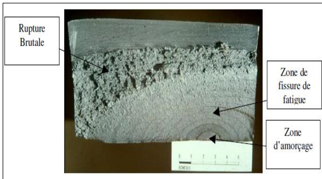
Figure 45: Faciès de la rupture [66]
