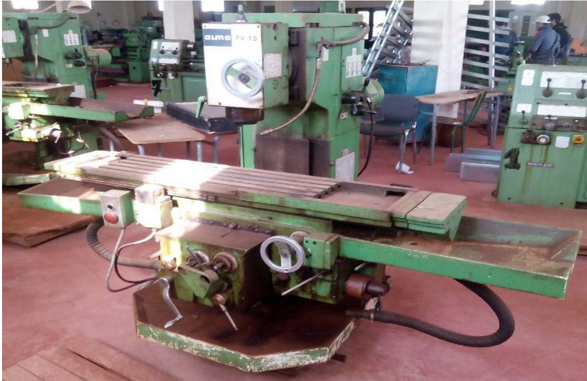
Figure I.8 Fraiseuse verticale PMO FV 2.5
