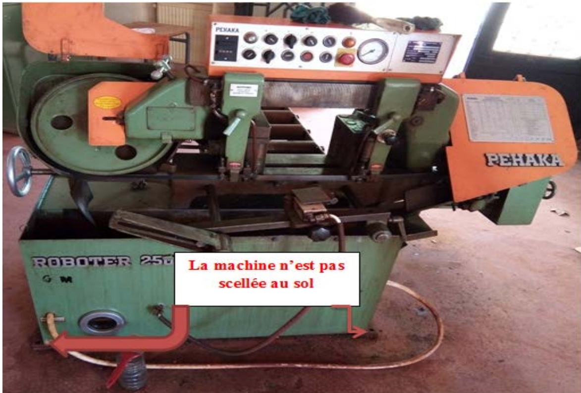
Figure III.4.3 - Machine non scellée au sol.
