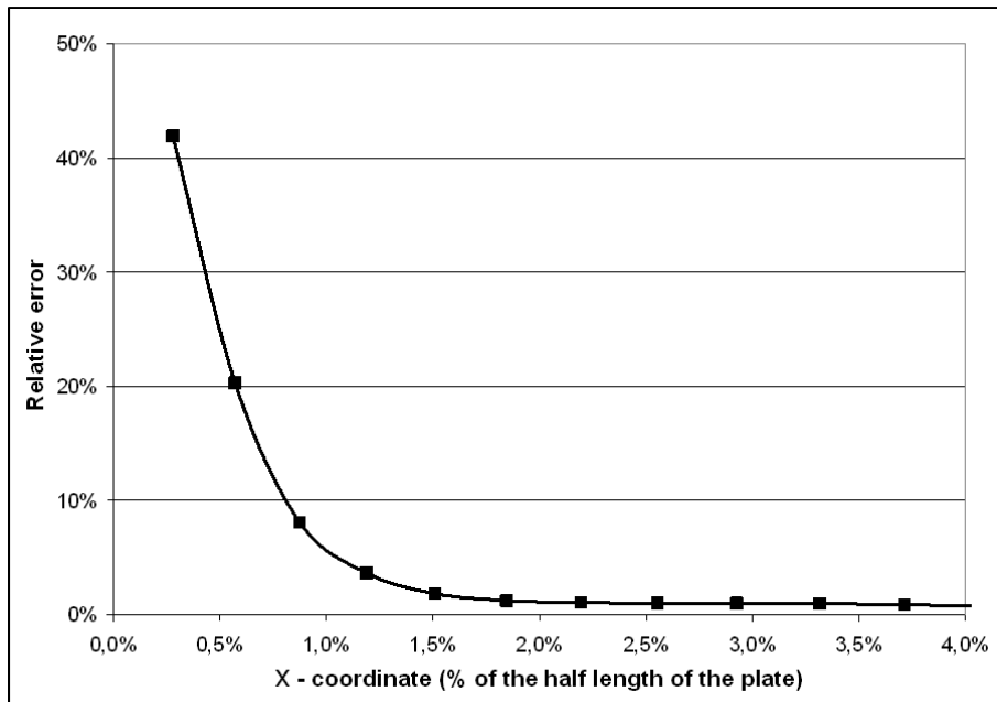
Figure 2.11 Relative error between the half and complete models as a function of x-coordinate (plane of symmetry is at x = 0 )
