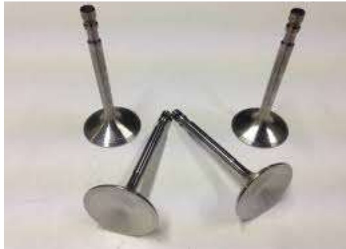
Figure 1.12 : Soupape admission Gordien[5].
