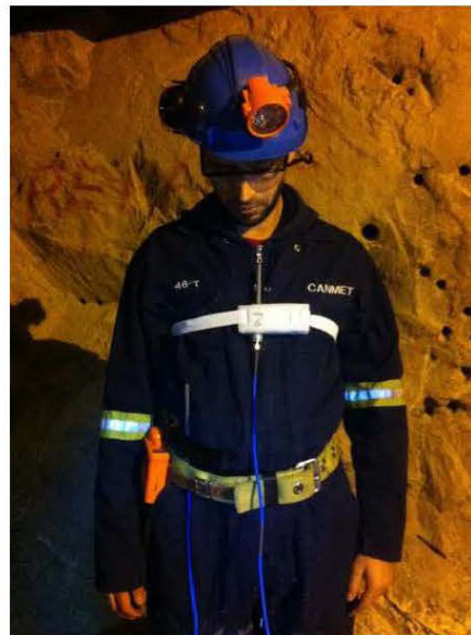
Figure 6- 5. On-body measurements test set up in a mine gallery
