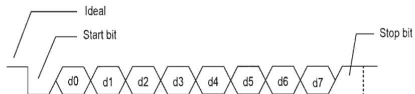
Figure 4-3 UART serial bit structure
