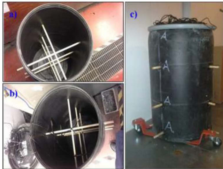
Figure 5-4: Instrumented barrel with RT-1 sensors before (a and b) and during the test (c)
