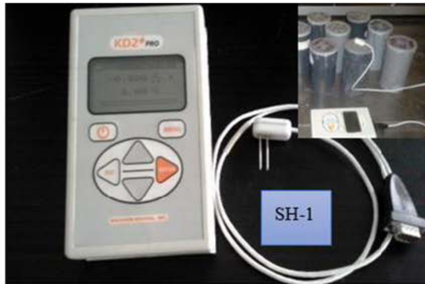
Figure 4-2 : Photo of Molded backfills showing thermal properties measurements using KD2 Pro analyser
