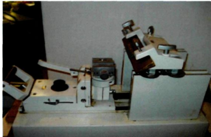
Figure 4.3: Microtome Leitz Wetzlar
