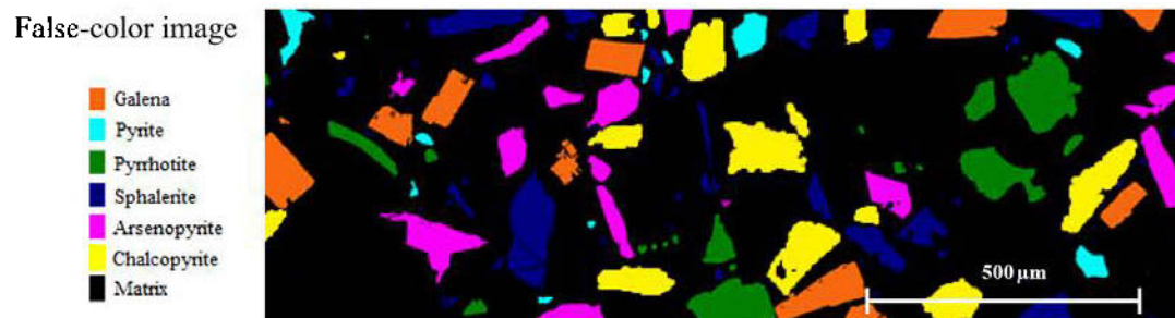
Figure 6.12 False-color image processed by Clemex Vision PE® using I436, I480 and I605
