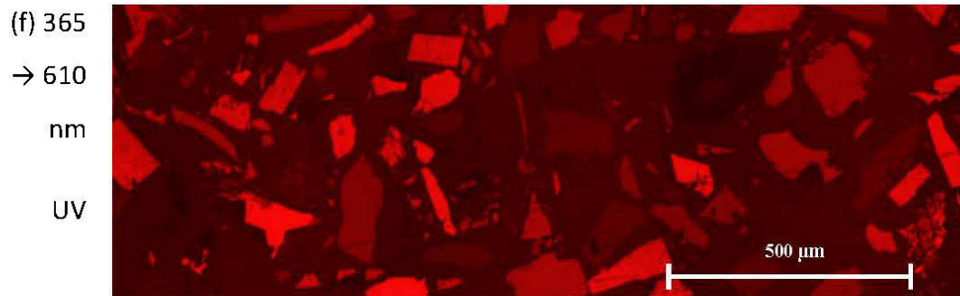
Figure 6.3 Stitched images, (a) in white light and acquired with the excitation filters at (b) 436, (c) 480, (d) 605 and (e) 650 nm. (f) UV image, acquired after conversion into a visible 610 nm image
