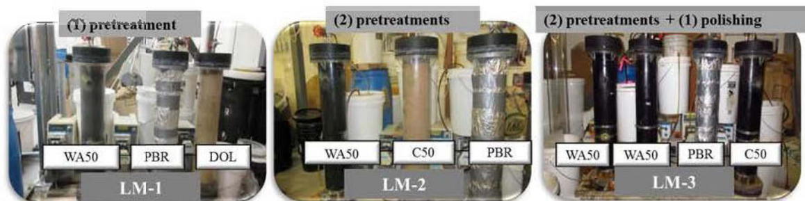
Figure C.1 Configuration of the three scenarios (LM-1, LM-2, LM-3) of multi-step systems during laboratory experiments
