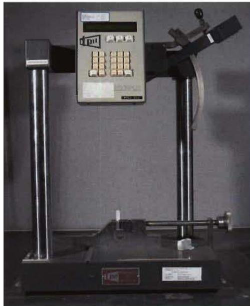
Figure 19: Machine d'impact TMI ([www.testingmachines.com](http://www.testingmachines.com))
