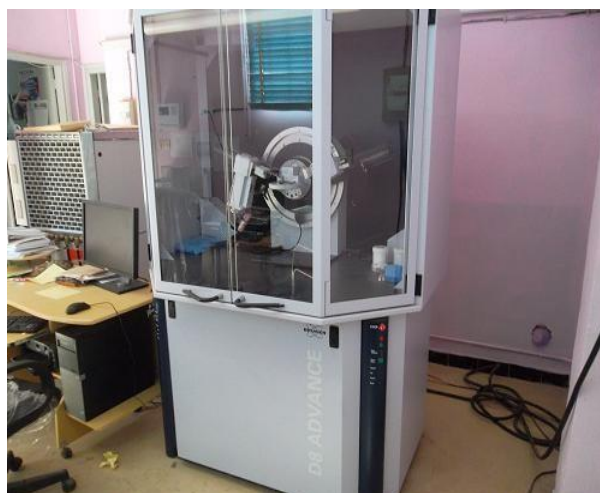
Figure 2 : Diffractomètre de rayons X, Bruker AXS D8 Advance (LCP, Oran).
