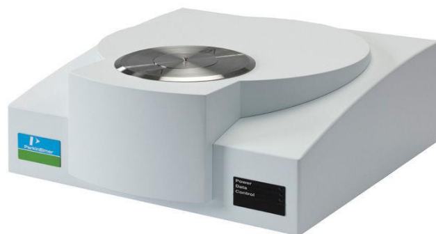
Figure 6 : ATG Perkin Elmer STA 6000
