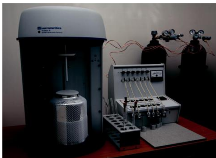
Figure 13 : Appareil BET TriStar 3000.
