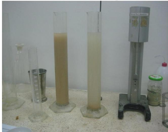
Photo 3.22 double hydrometer test
