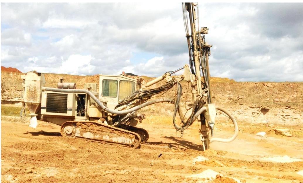
*Figure 15: Machine hydraulique foreuse*
