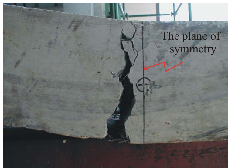
Figure 3-7: photo shows the failure mode for the tested beams.
