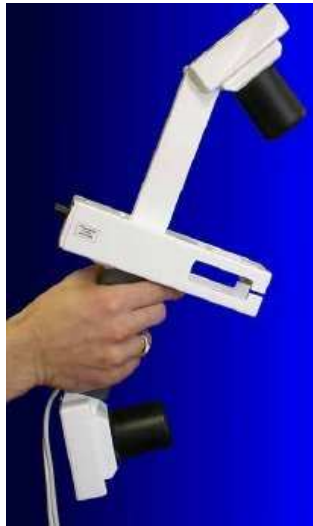
Figure 2.4: The Polhemus laser scanner.
