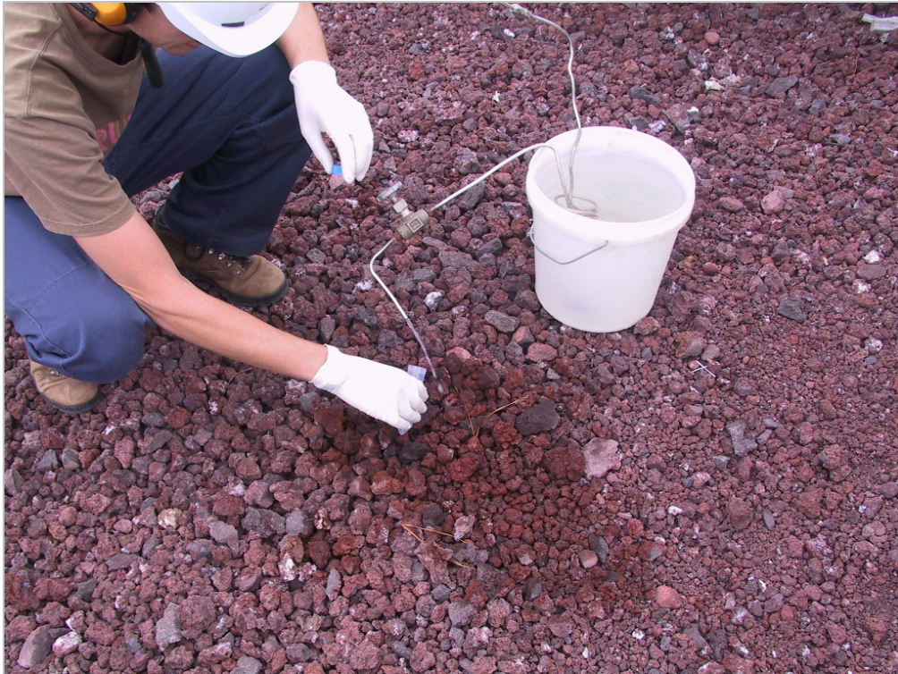
Plate 2.1 Cooling coil used to collect power station fluids, shown with the coil passing through a bucket of cold water before sample collection.
