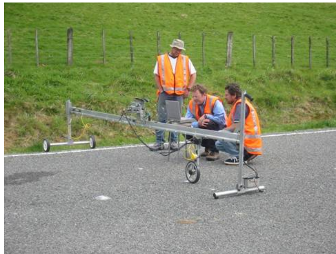
Figure 4.9: Transverse Profile Beam
