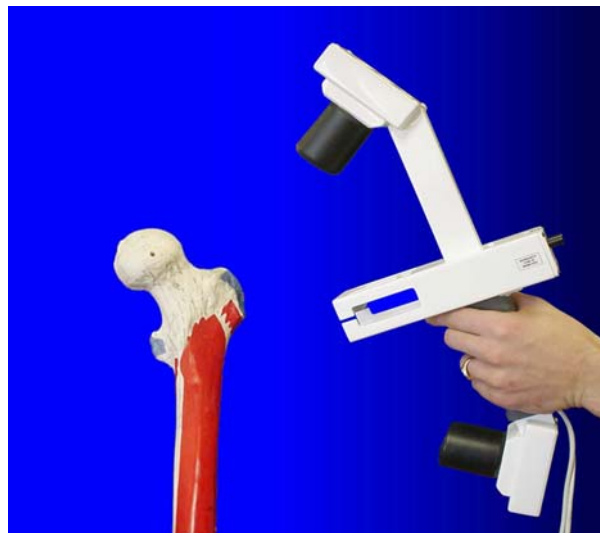
FIGURE 4.10: The Polhemus FastScan™ Laser Scanner used to validate the host mesh method.
