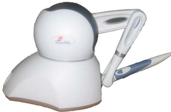
FIGURE 2.4: The Phantom® Omni™ haptic device senses 6 degrees of freedom, and can produce a force with 3 degrees of freedom.
