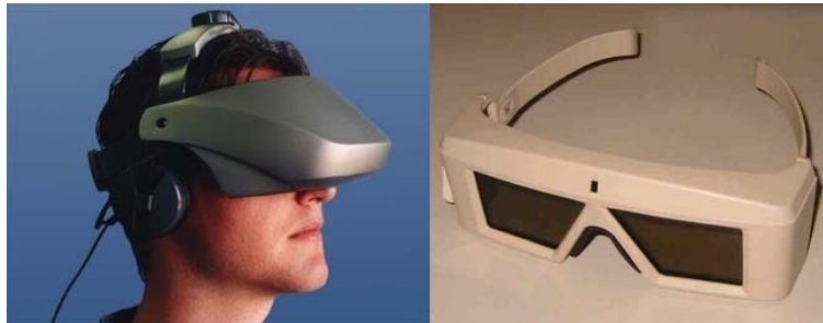
FIGURE 2.15: The 5DT HMD 800 head mounted display and LCD shutter-glasses. Accessed at http://www.5dt.com
