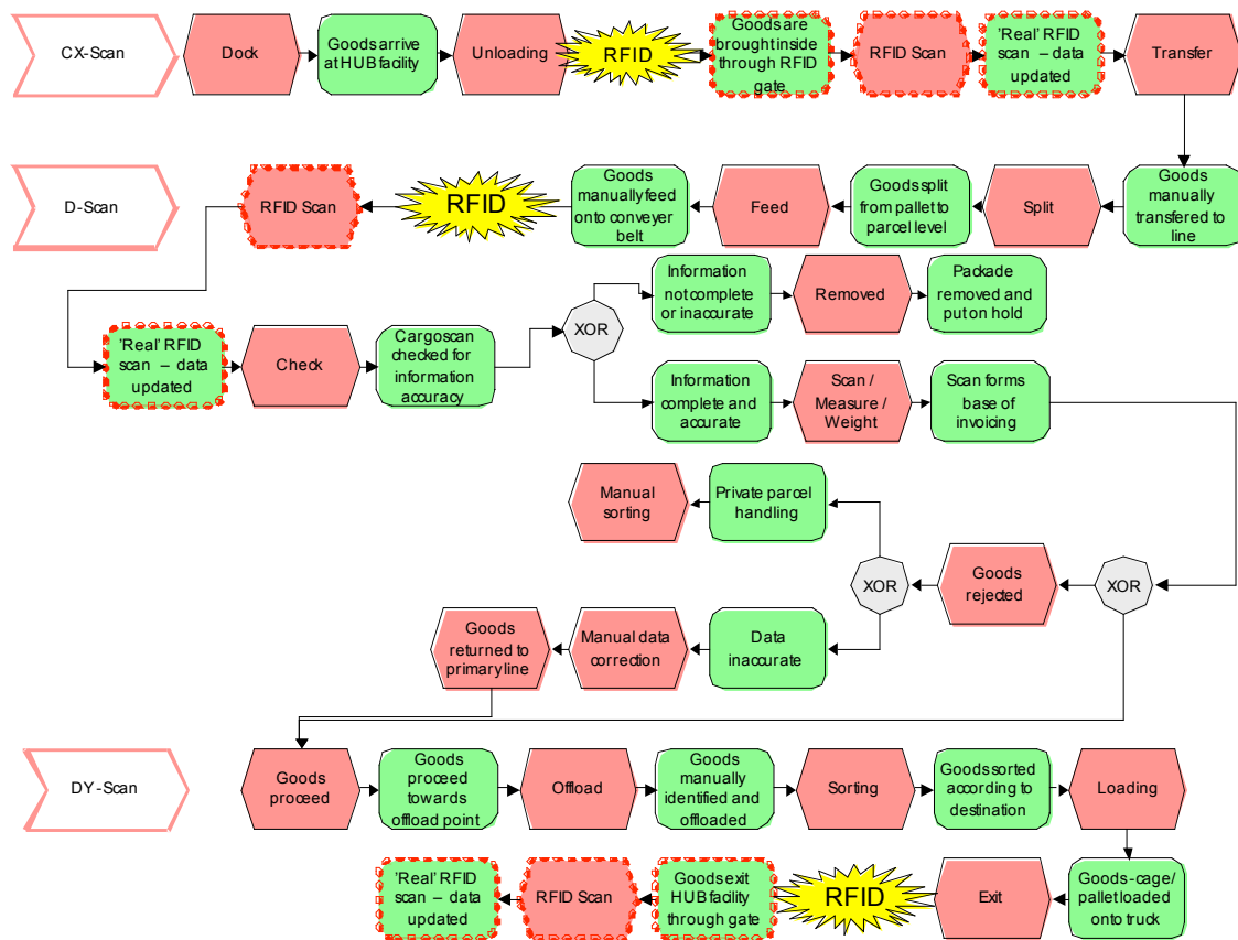
Figure 7 Proposed goods flow process after RFID implementation
