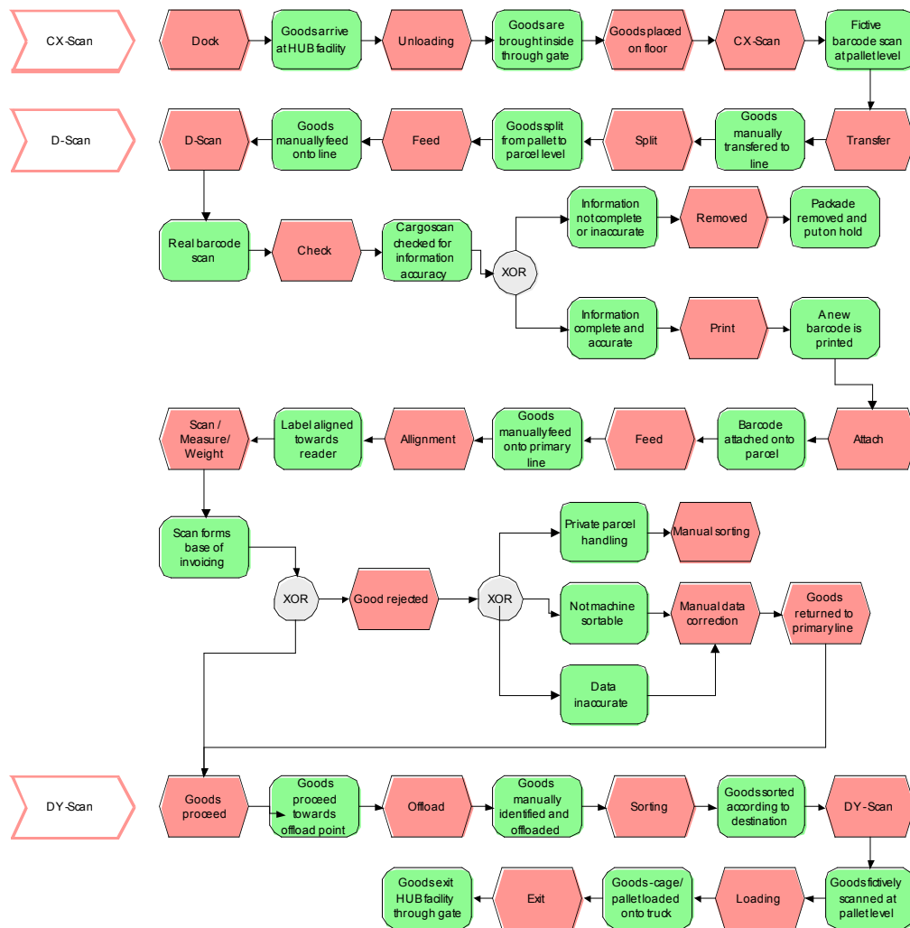
Figure 6 Current goods flow process of the HUB in Jönköping
