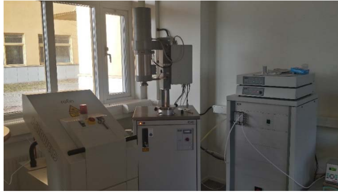
Figure 20. A laser flash apparatus, Netzsch LFA 427, used to determine the thermal diffusivity.
