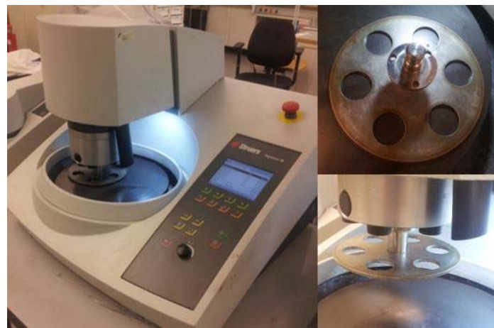
Figure 33. Equipment used for grinding and polishing, Struers Tegramin-30 with a sample holder for six samples.
