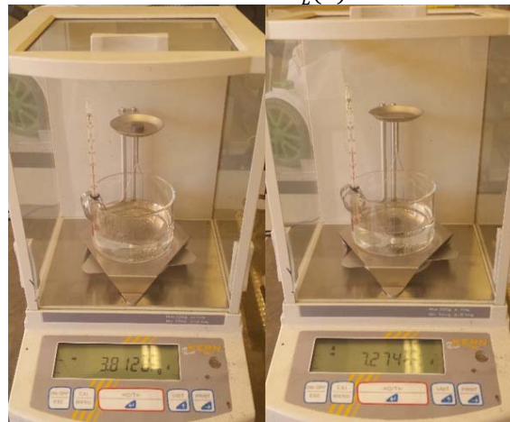
Figure 17. An analytical balance used to determine density by weighing a sample first in air (left picture) and then in water (right picture).
