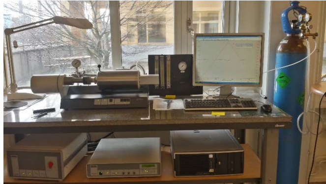
Figure 16. A Netzsch DIL 402C push-rod dilatometer used to measure thermal expansion.
