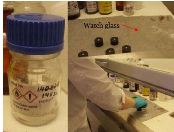
Figure 34. Etching procedure consisting of immersing samples in a 2 % Nital solute.
