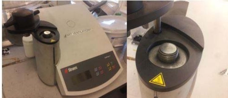
Figure 30. Embedding equipment used, Struers citopress-1 with a close up on the cylindrical piston to put the sample.
