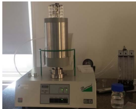
Figure 19. A DSC machine, Netzsch DSC 404 C, used to determine the specific heat.
