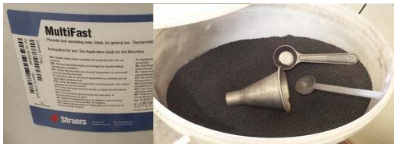
Figure 31. Multifast, the phenolic hot mounting resin used.
