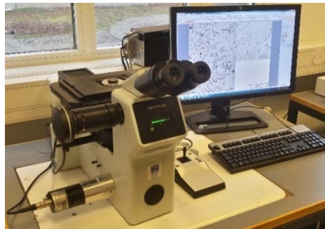
Figure 35. The optical microscope, Olympus GX71, used to capture images of the microstructure.
