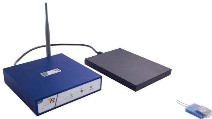
Fig. 1-5: A TET charging base and an implantable biomedical sensor [61]
