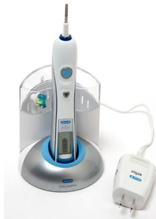
Fig. 1-3: Wireless charging electric toothbrush [33]
