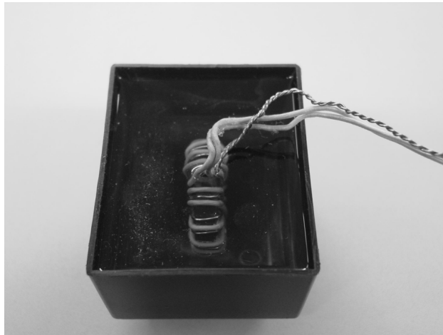
Fig. 6.14 The potted 30x18x6 mm CUT
