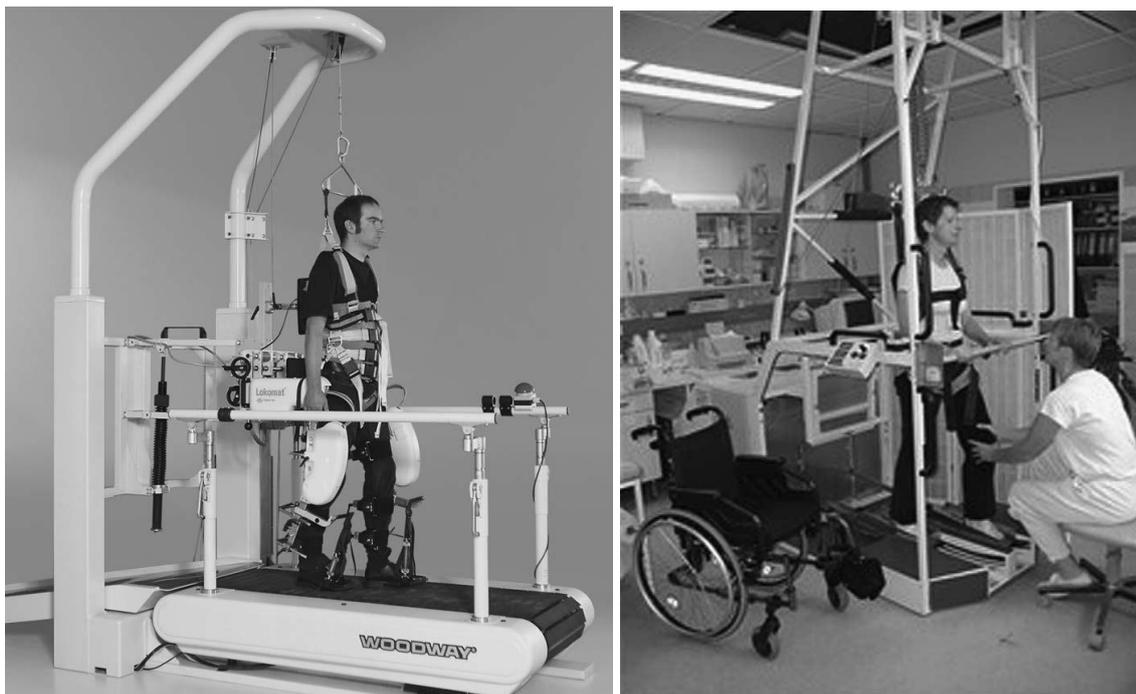
**Figure 1-1 Left: Lokomat, a treadmill based exoskeleton type of gait rehabilitation robot. (Reproduced from [9] © 2011 IEEE). Right: Gait Trainer, an end-effector gait rehabilitation robot. (Reproduced from [10] Copyright © 2007 SAGE Publications)**
