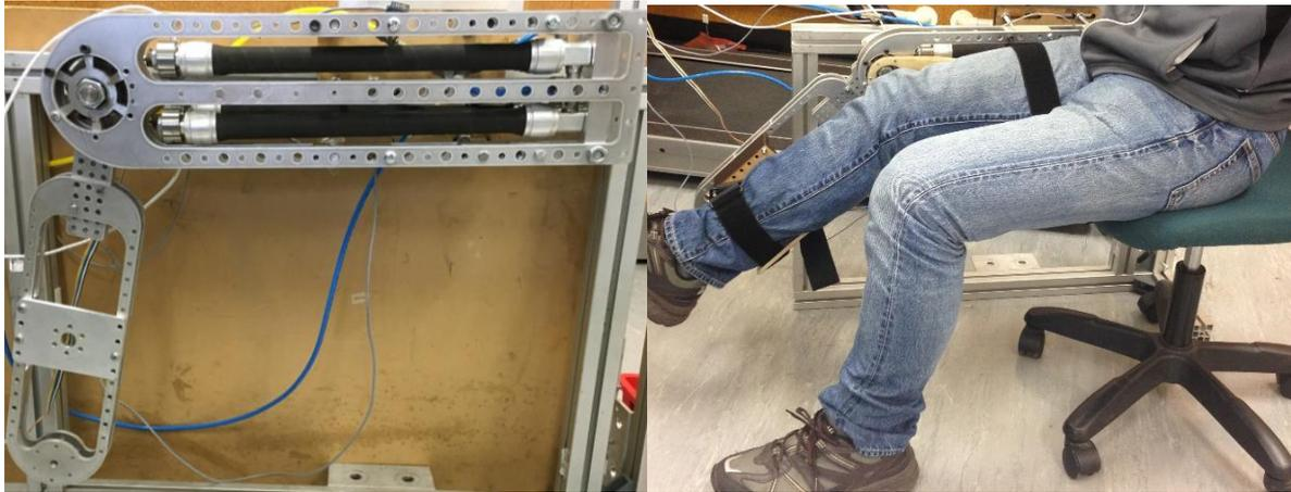
**Figure 5-2 Left: structure of the knee joint mechanism; right: a healthy subject participating validation experiment with the mechanism**
