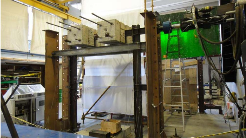
Figure 3-14 Steel moment resisting frame specimen (MRF) used in the experimental validations
