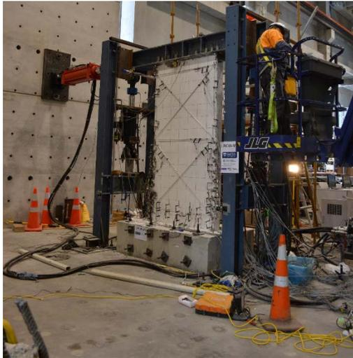
a) Photo from actual test setup of the quasi-static and hybrid simulation without substructuring
