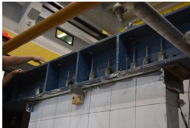
c) Connection between top of the wall and loading beam
