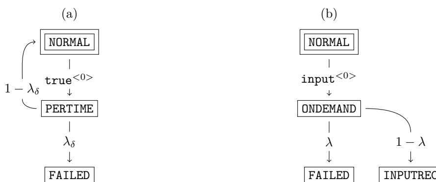
Figure 6.9: Modelling (a) per-time and (b) on-demand probabilistic failures
