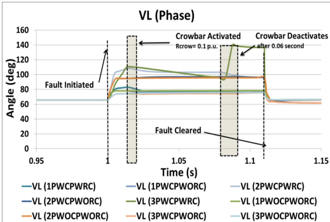
Figure 7.9: Line to ground voltage phase
