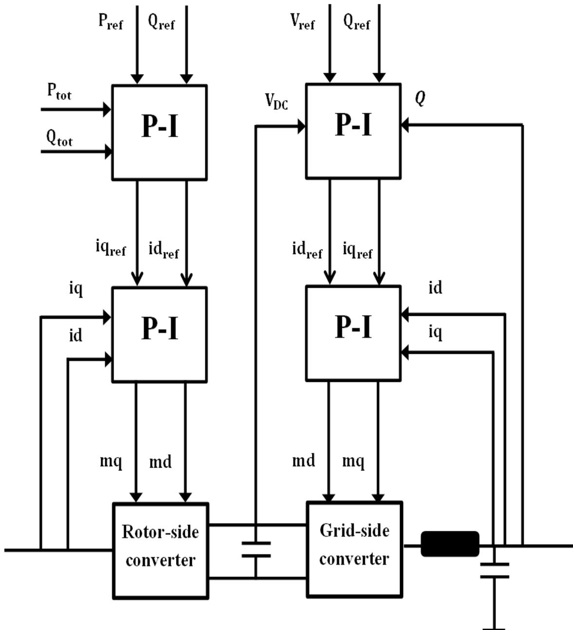
Figure 7.5: Electrical control-scheme of the DFIG
