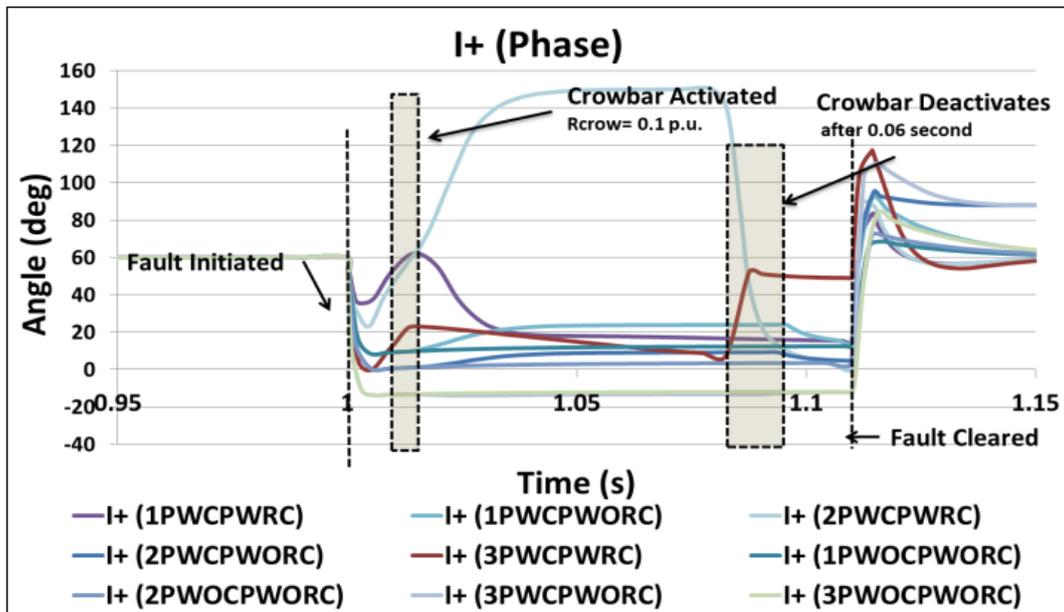
Figure 7.18: Positive sequence current phase
