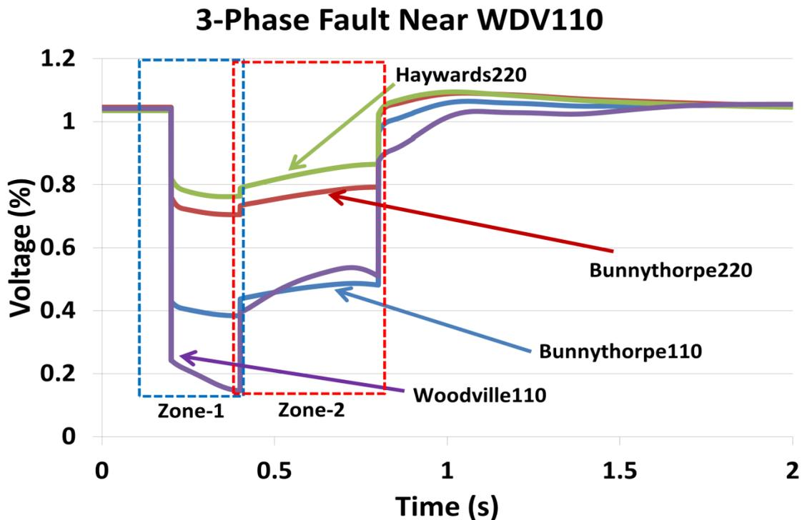
Figure 5.8: A 3-phase symmetrical fault near WDV110
