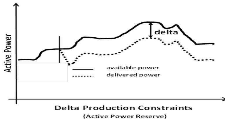
Figure 2.5: Delta Production Constraint
