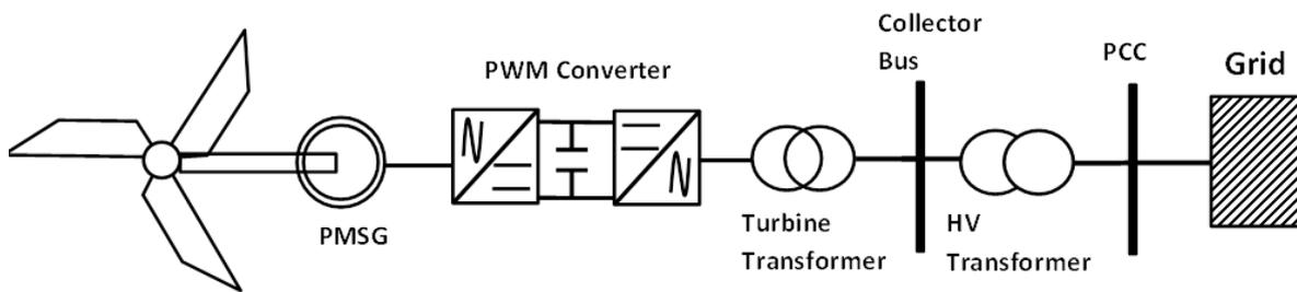
Figure 3.1d: Full Scale Frequency Converter (FSFC) Permanent Magnet Synchronous Generator (PMSG) Wind Turbine (Type-4)
