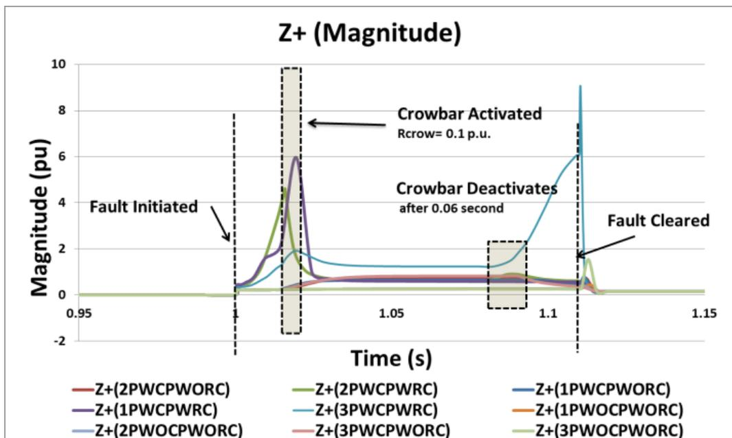
Figure 7.21: Positive sequence impedance magnitude
