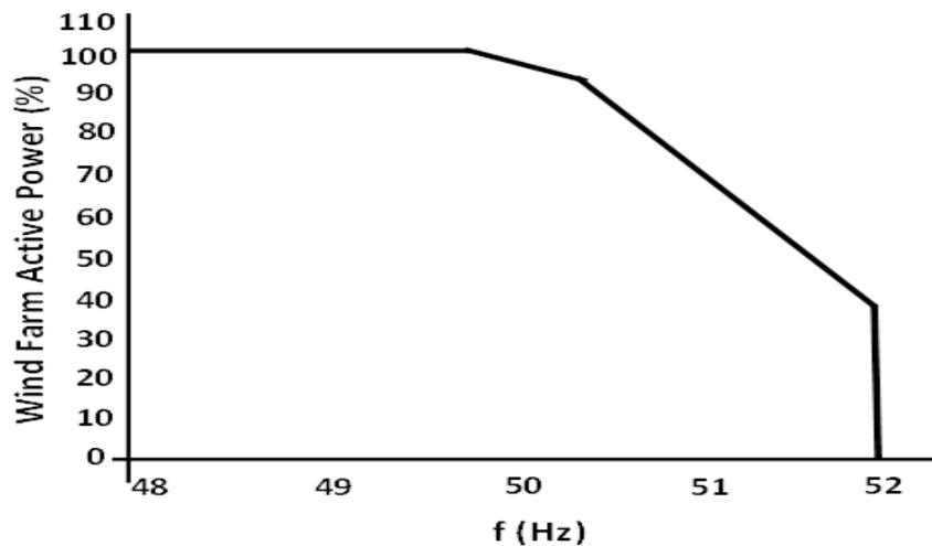
Figure 2.7: Typical power-frequency response curve
