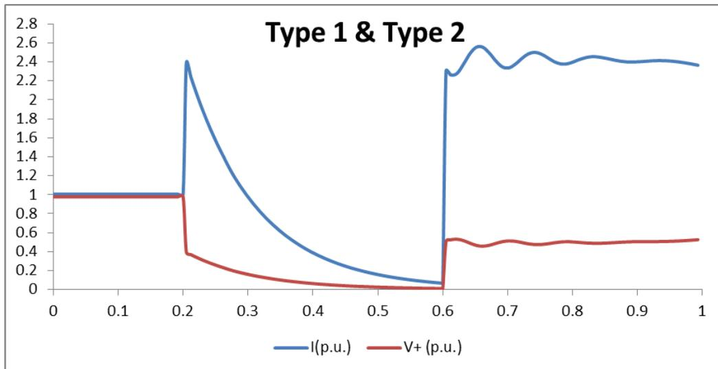
Figure 6.8: Fault Response of Types 1 &amp; 2 (IG) Wind Farms
