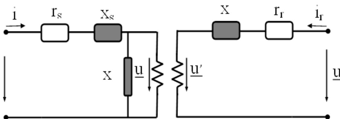
Figure 7.1: Equivalent circuit of the DFIG
