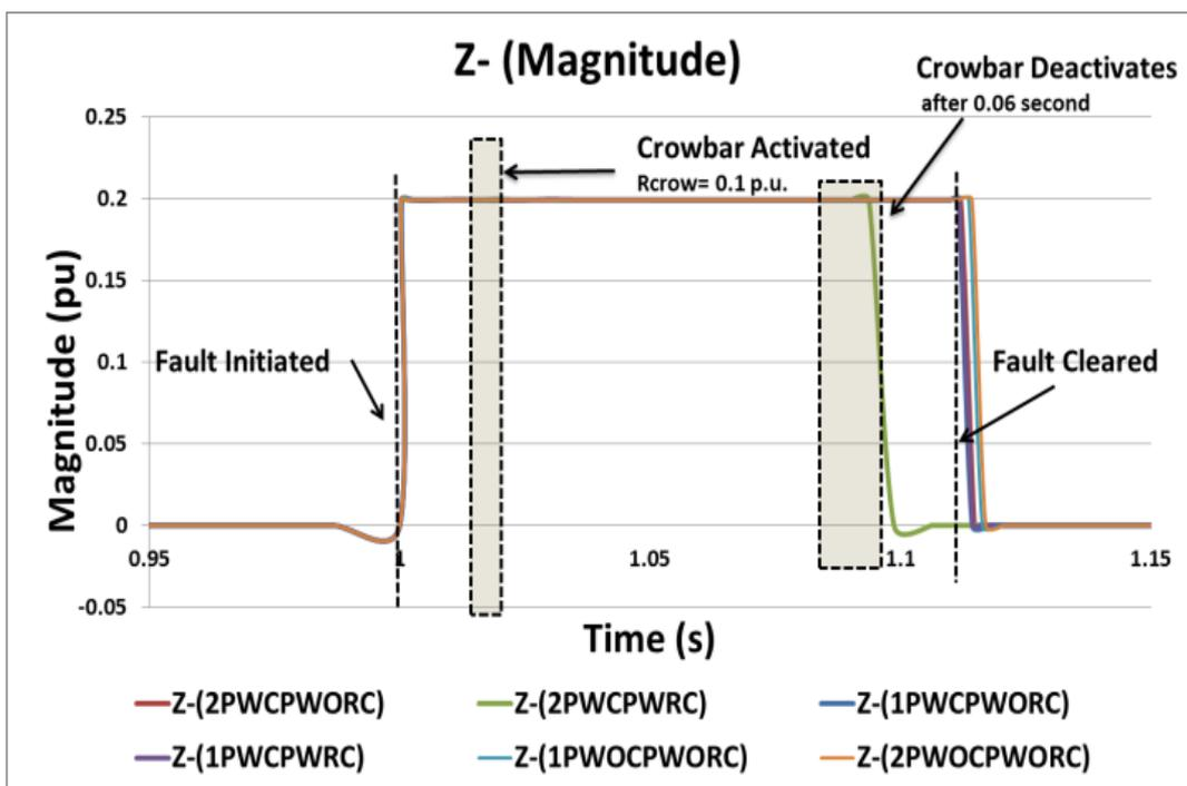
Figure 7.23: Negative sequence impedance magnitude
