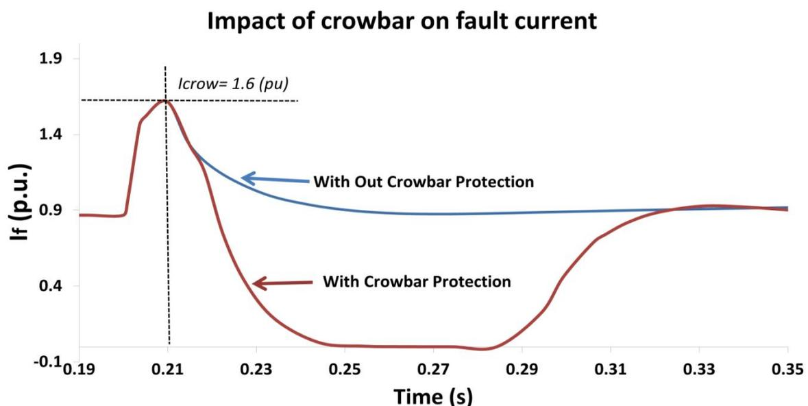
Figure 6.7: Impact of crowbar duration on fault current
