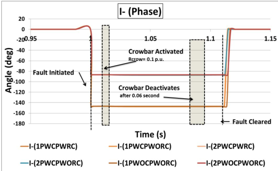
Figure 7.20: Negative sequence current phase
