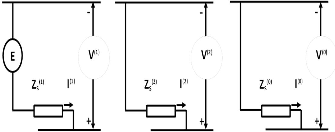
Figure 7.6: Deriving fault models
