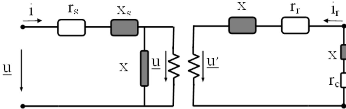
Figure 7.2: DFIG with inserted crowbar protection ( $r_c$  and  $x_c$ )
