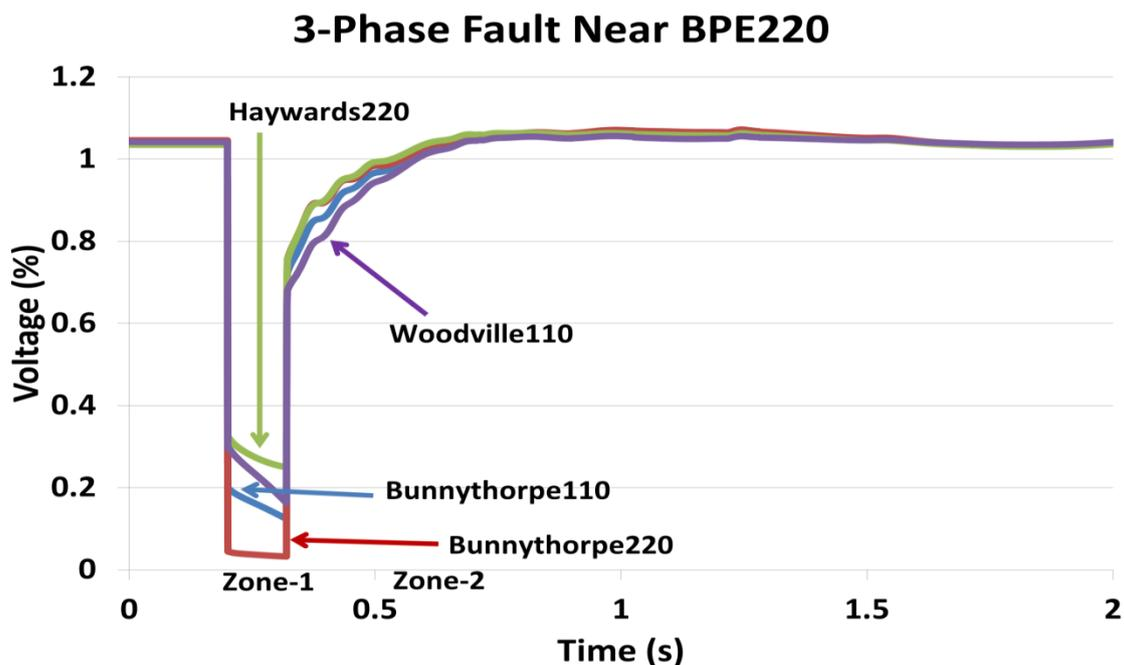
Figure 5.10: A 3-phase symmetrical fault near BPE220
