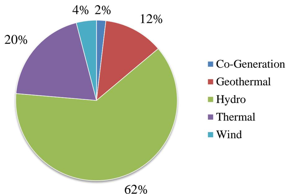
Figure 2.10: Typical New Zealand Generation Mix
