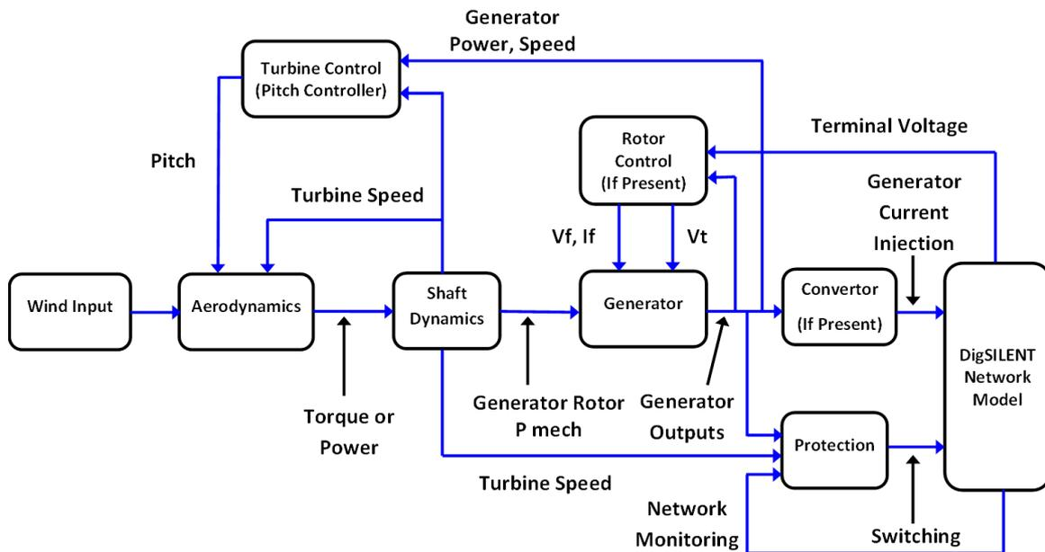
Figure 3.2: General structure of a wind generator model
