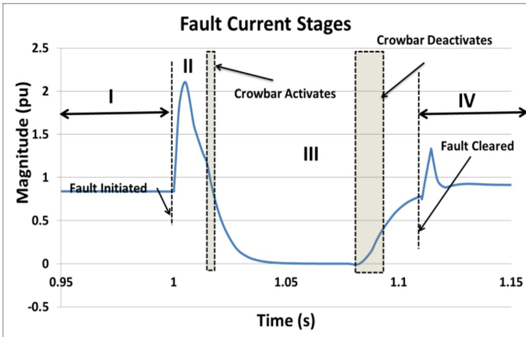
Figure 7.12: Fault characteristics DFIG-based large wind farms
