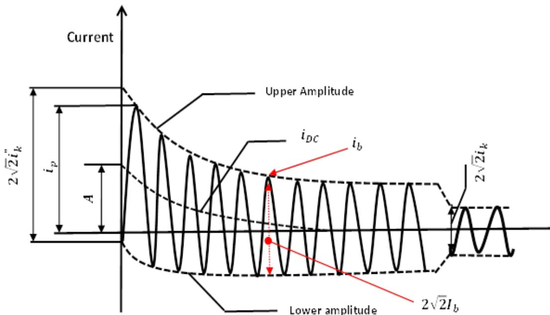
Figure 4.2: Short-Circuit Current Time Function
