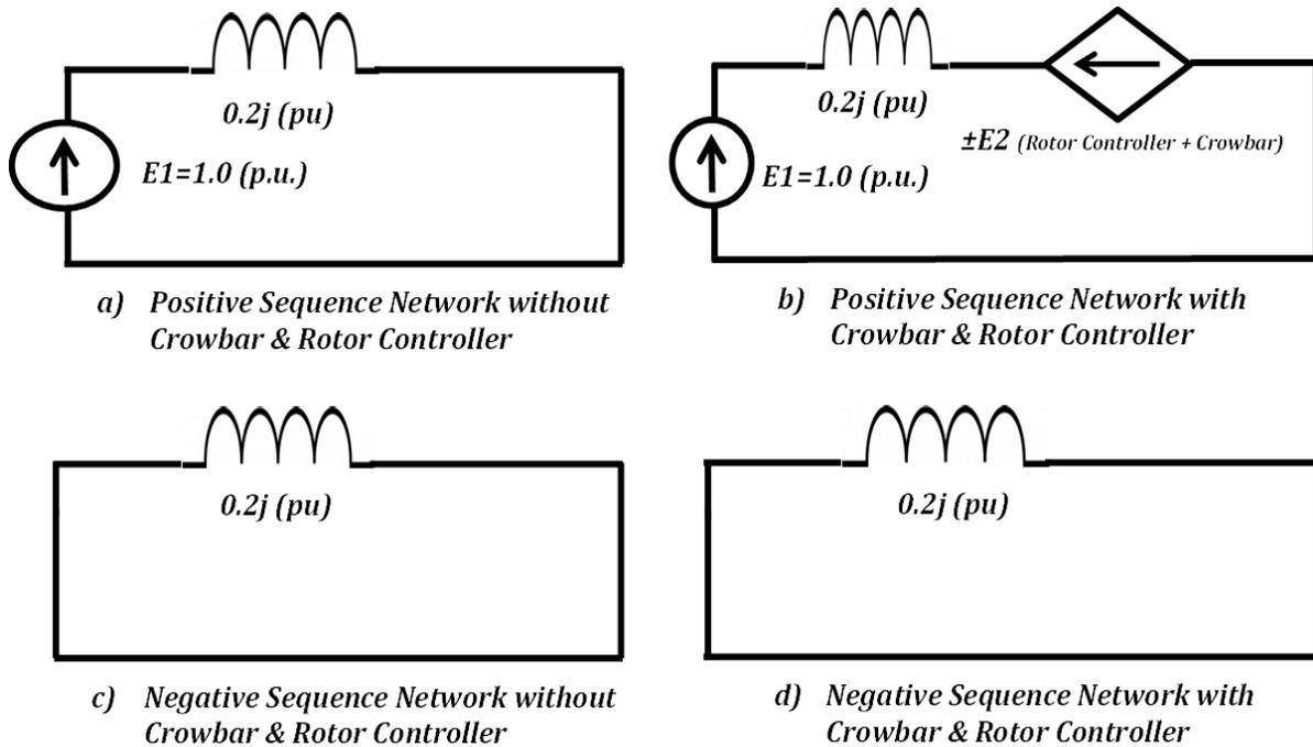
Figure 7.25: SNEs for DFIG-based Large Wind farm
