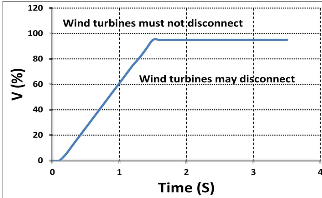
Figure 5.1: Typical limit curve for LVRT requirements
