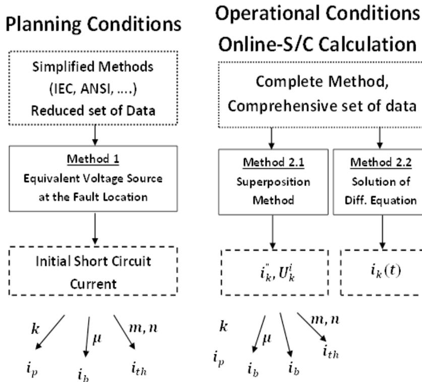
Figure 4.1: Areas of Application of Short-Circuit Calculations
