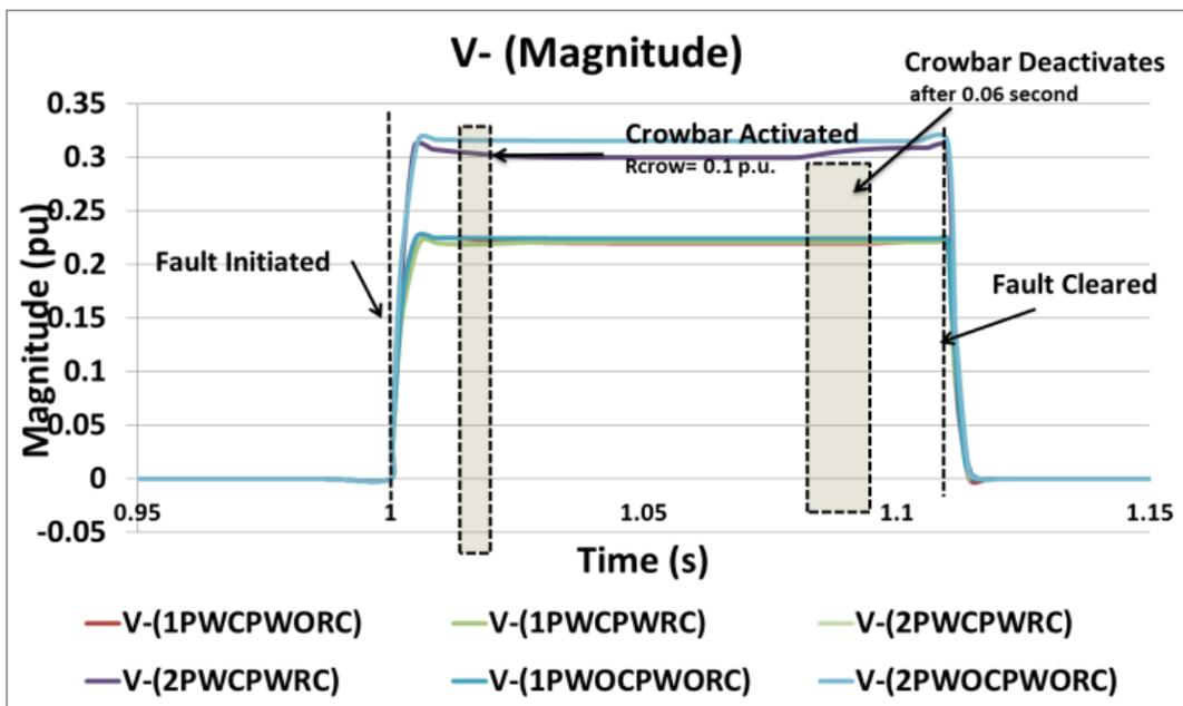
Figure 7.15: Negative sequence voltage magnitude
