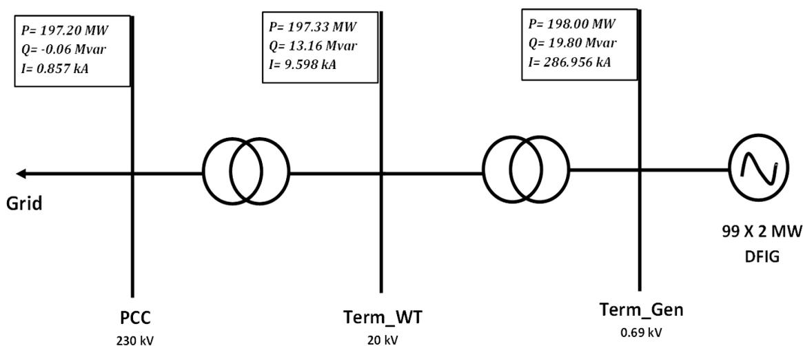
Figure 7.7: Simulation setup of a DFIG-based wind farm
