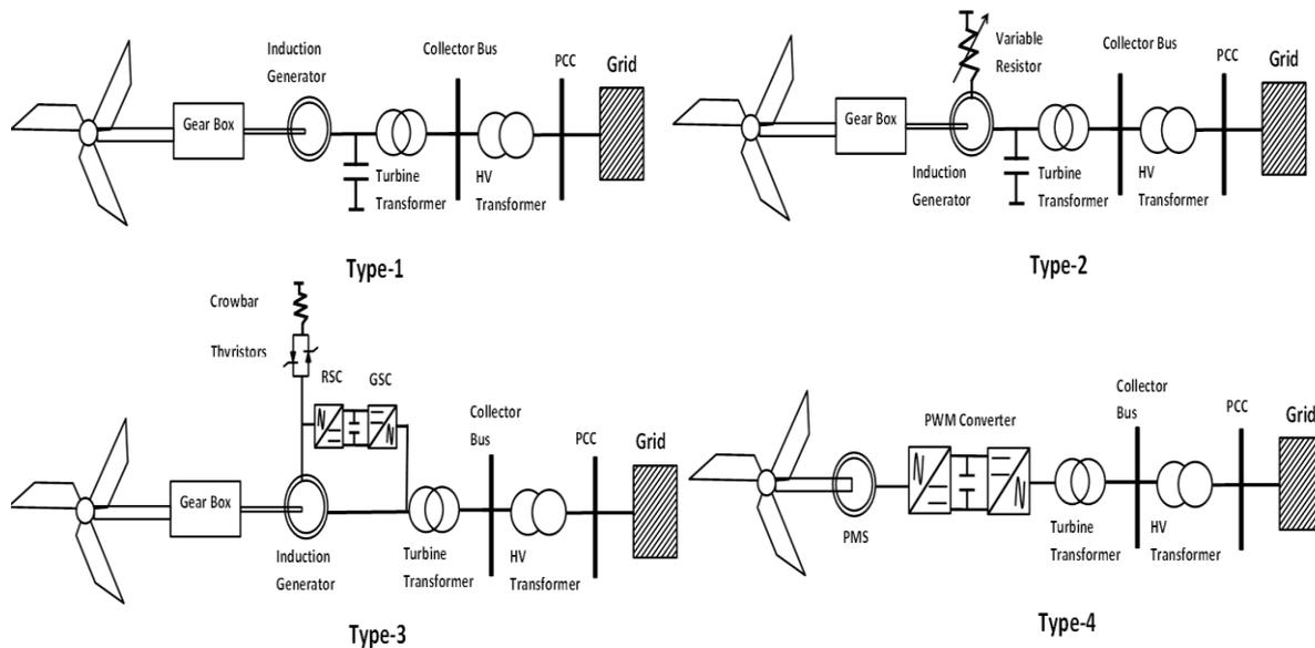
Figure 2.8: Wind Turbine Generator (WTG) Types
