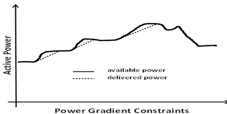
Figure 2.6: Power Gradient Constraint
