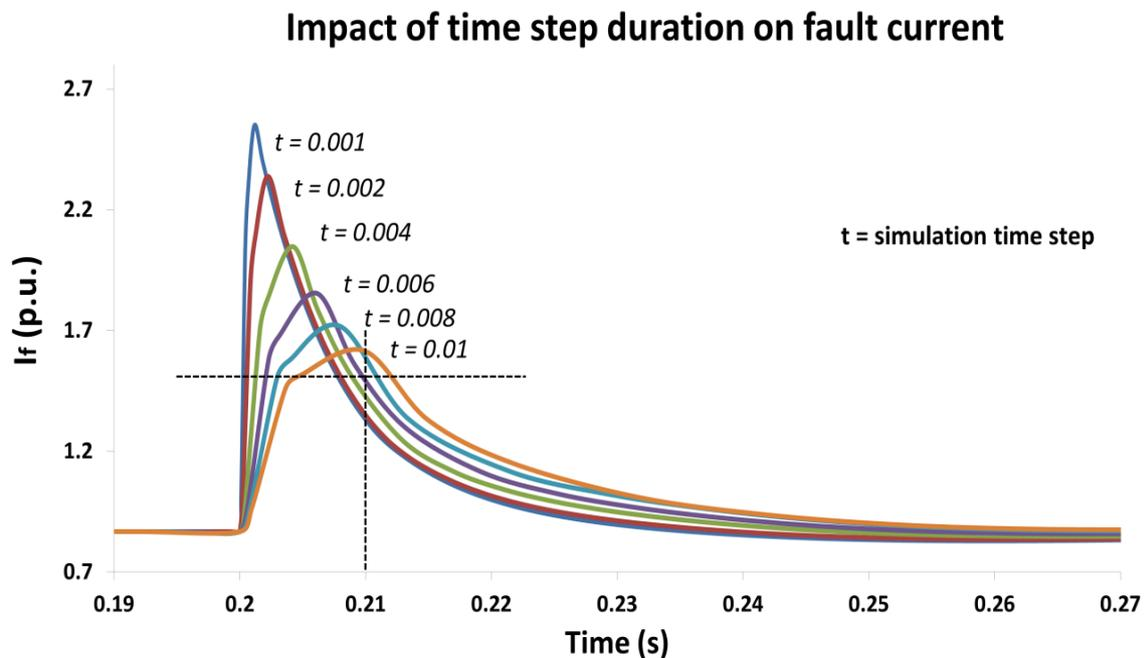
Figure 6.6: Impact of time-step duration on fault current
