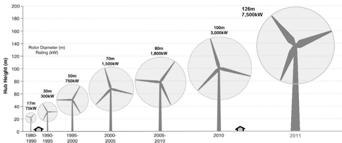
Figure 2.2: Wind Turbine Sizes and Capacities
