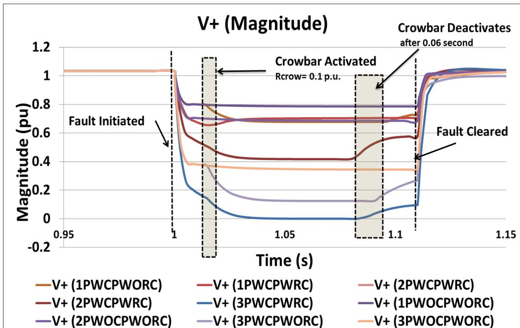
Figure 7.13: Positive sequence voltage magnitude
