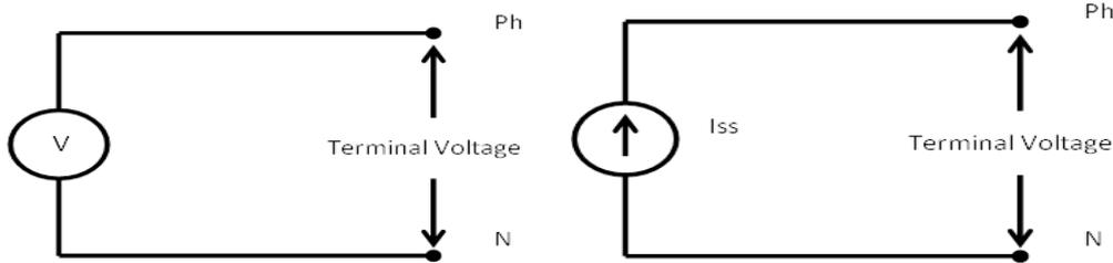
Figure 6.13a: Equivalent Circuit of Types 1, 2 &amp; 3 immediately After Fault
