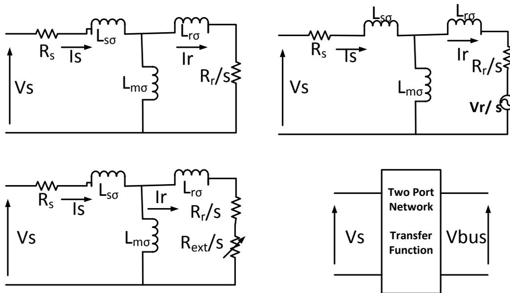
Figure 2.9: Wind Turbine Generator (WTG) Equivalent Models
