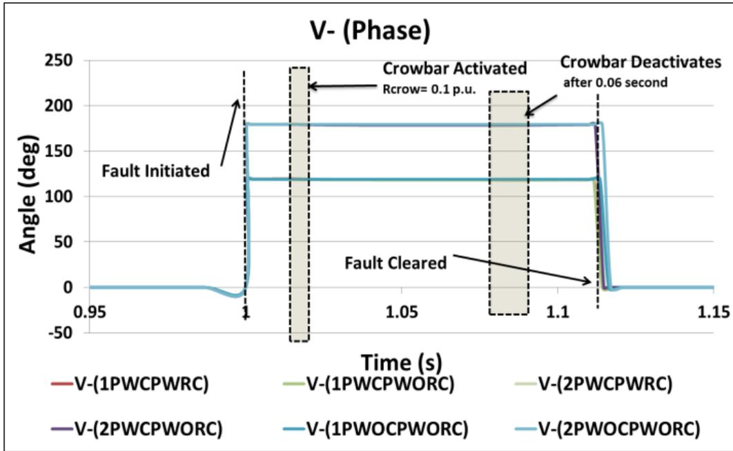
Figure 7.16: Negative sequence voltage phase
