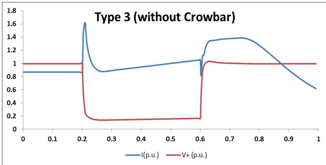
Figure 6.10: Fault Response of Type-3 WTG without Crowbar
