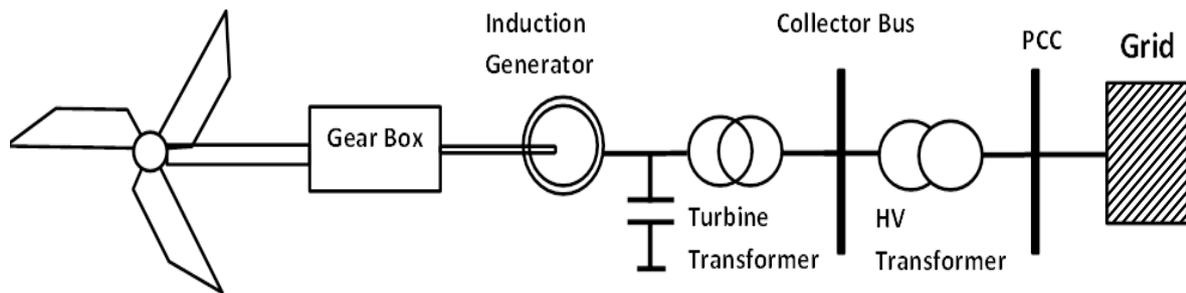
Figure 3.1a: Squirrel Cage Induction Generator (SCIG) Wind Turbine (Type-1)
