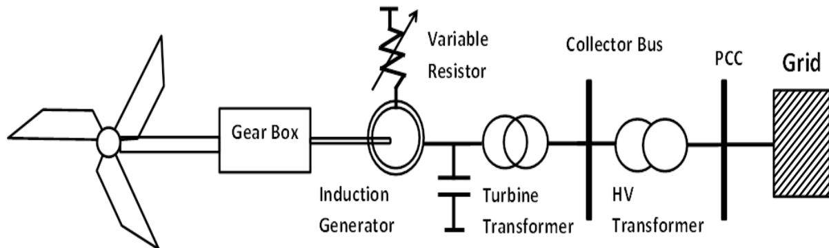
Figure 3.1b: Wound Rotor Induction Generator (WRIG) Wind Turbine (Type-2)
