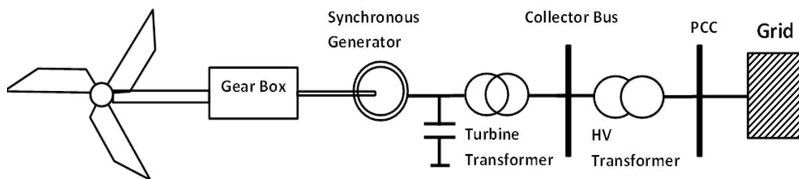
Figure 5.3: Type-5 Wind Turbine Generator
