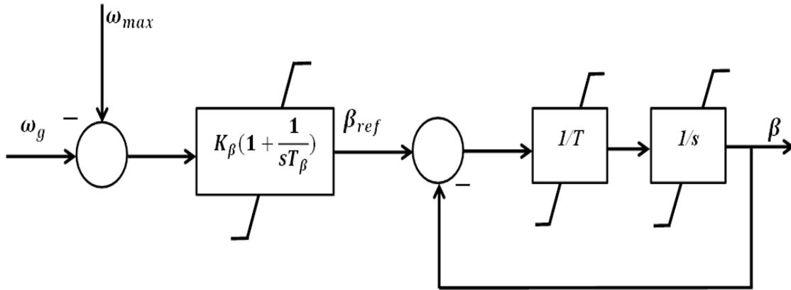
Figure 7.4: Generic model of the pitch control system
