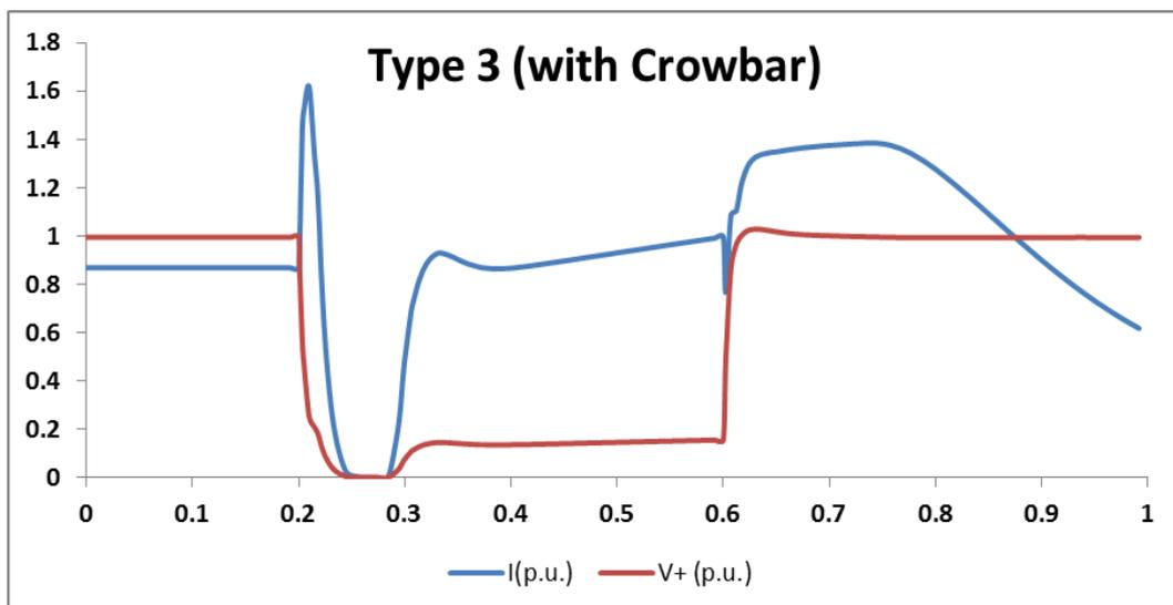
Figure 6.9: Fault Response of Type-3 WTG with Crowbar
