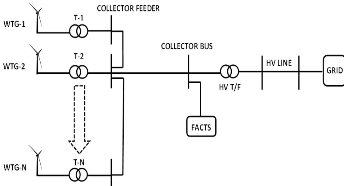
Figure 6.2: Wind Farm Interconnection with Grid
