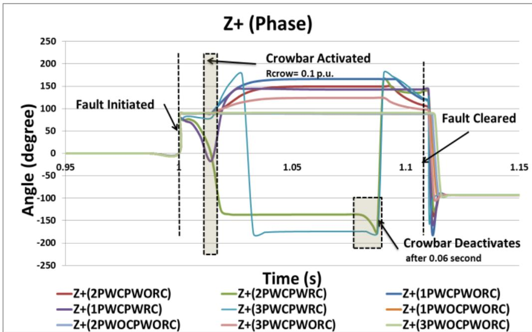
Figure 7.22: Positive sequence impedance phase
