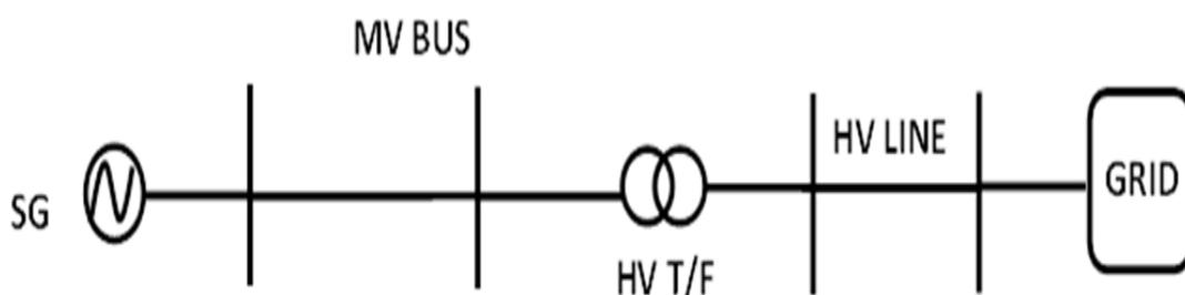
Figure 6.1: Conventional Generation Interconnection with Grid
