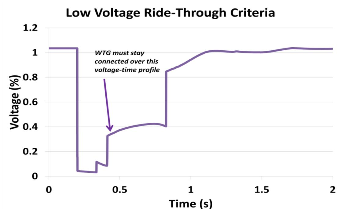
Figure 5.11: LVRT Criteria for Network under Study
