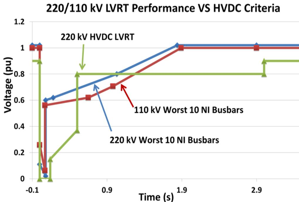
Figure 5.12: Summary and Existing HVDC Transpower Comparison – LVRT
