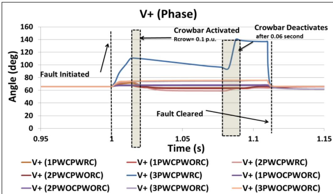
Figure 7.14: Positive sequence voltage phase
