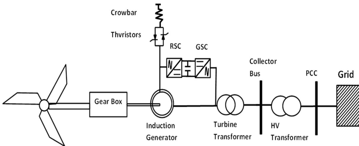
Figure 3.1c: Doubly Fed Induction Generator (DFIG) Wind Turbine (Type-3)
