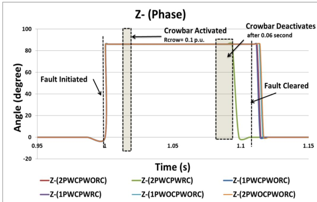
Figure 7.24: Negative sequence impedance phase
