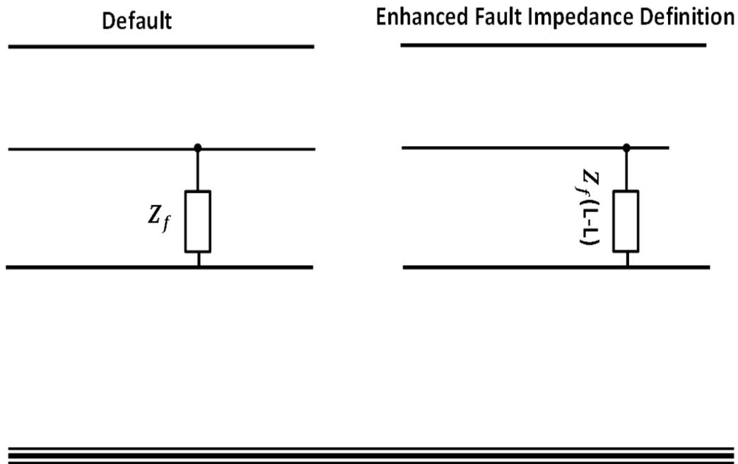
Figure 4.6: Fault Impedance Definition: 2-Phase Fault
