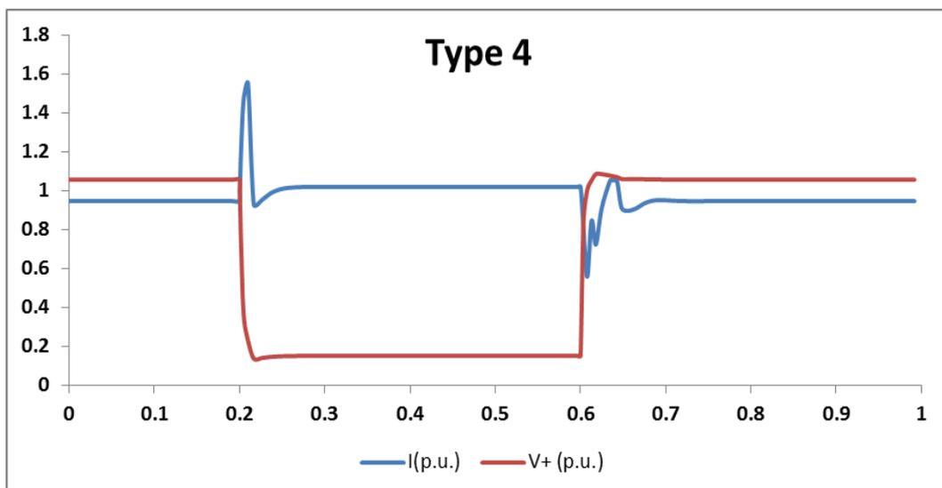
Figure 6.11: Fault Response of Type-4 WTG
