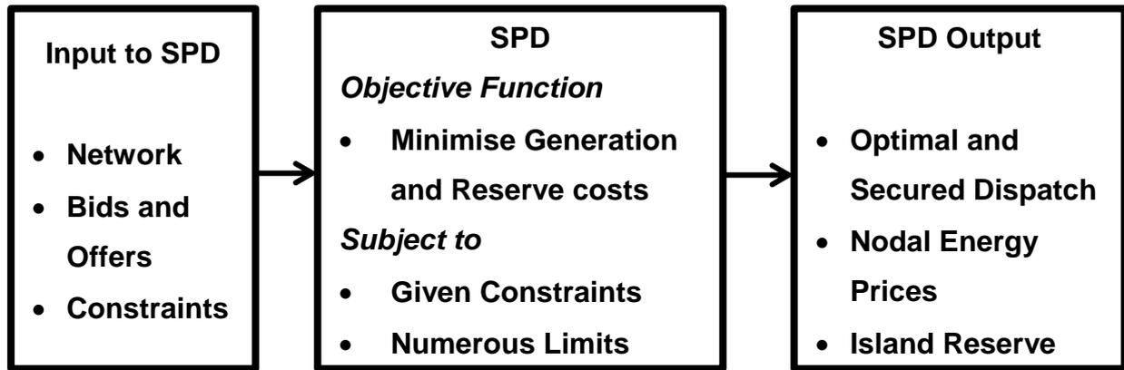
Figure 2.11: Functional Diagram of SPD
