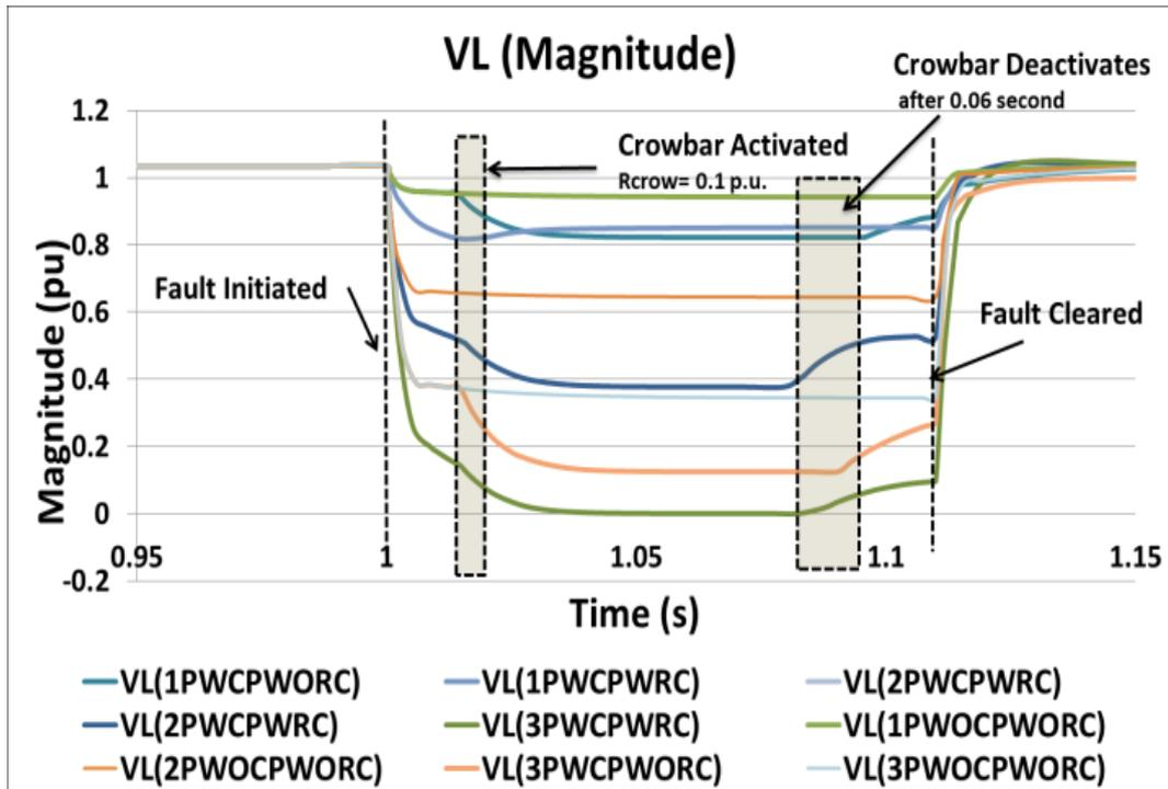
Figure 7.8: Line to ground voltage magnitude
