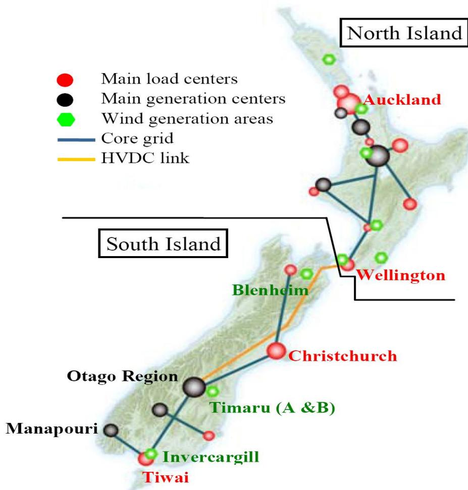
Figure 2.12: Transmission System in New Zealand [55]
