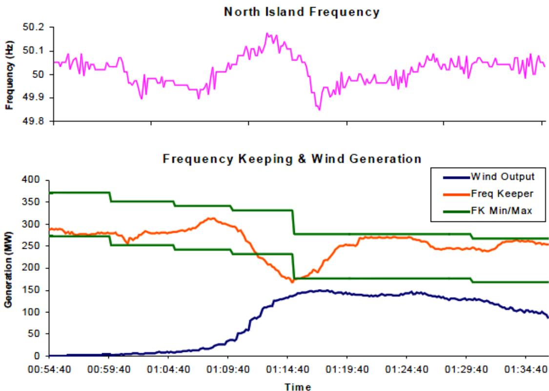
Figure 2.14: North Island frequency, frequency keeping generation (and frequency bands) in response to the events of 15 November 2004 [63]
