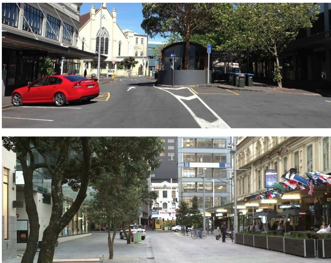
Figure 2.4 Road design and space allocation between a traffic-calmed street on Beresford Street (top) and a shared space on Fort Street (bottom) in Auckland, New Zealand.
