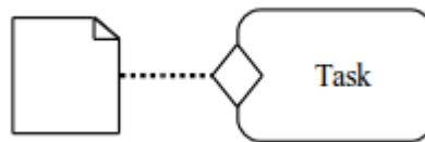
Figure 4.2: Event propagation notation between a case file item and a task
