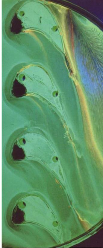
**Figure 6.11: Oil flow visualization of the endwall**
