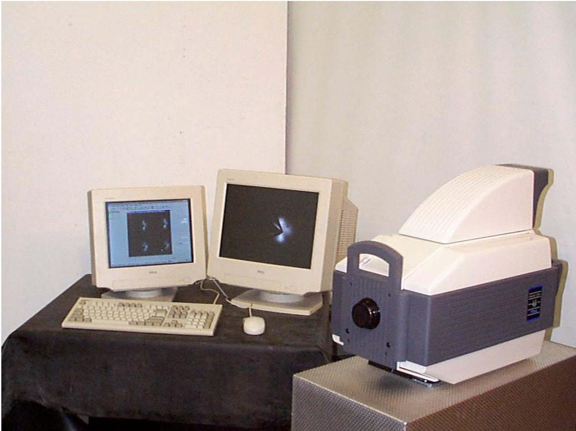
**Figure 3.2: Photograph of Imacon 468 Camera System**
