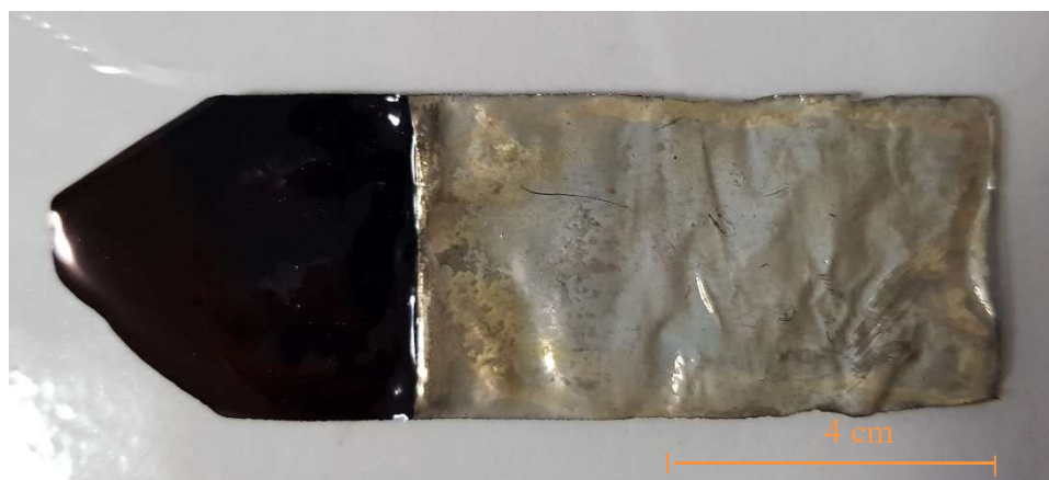
Figure 6.16: Photograph of a PANI film with metallic silver film after reaction of silver nitrate for >6 hours. The PANI to silver transition occurs due to the experimental set up, the PANI films were placed vertically in a beaker and the level of the solution is depicted by the transition.
