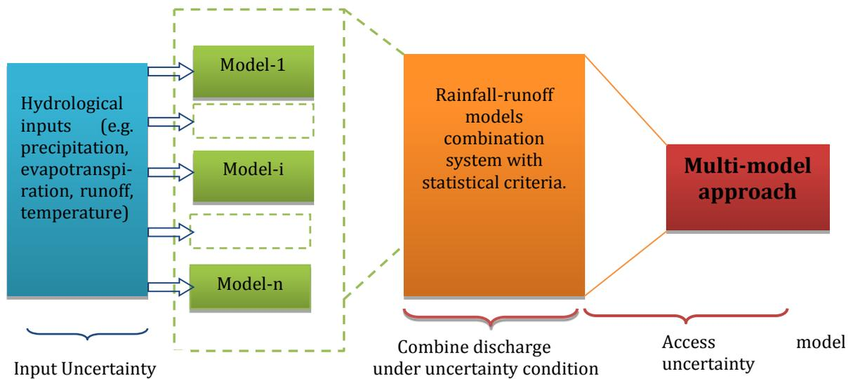
Figure 1.1: Schematic diagram of multi-model approach
