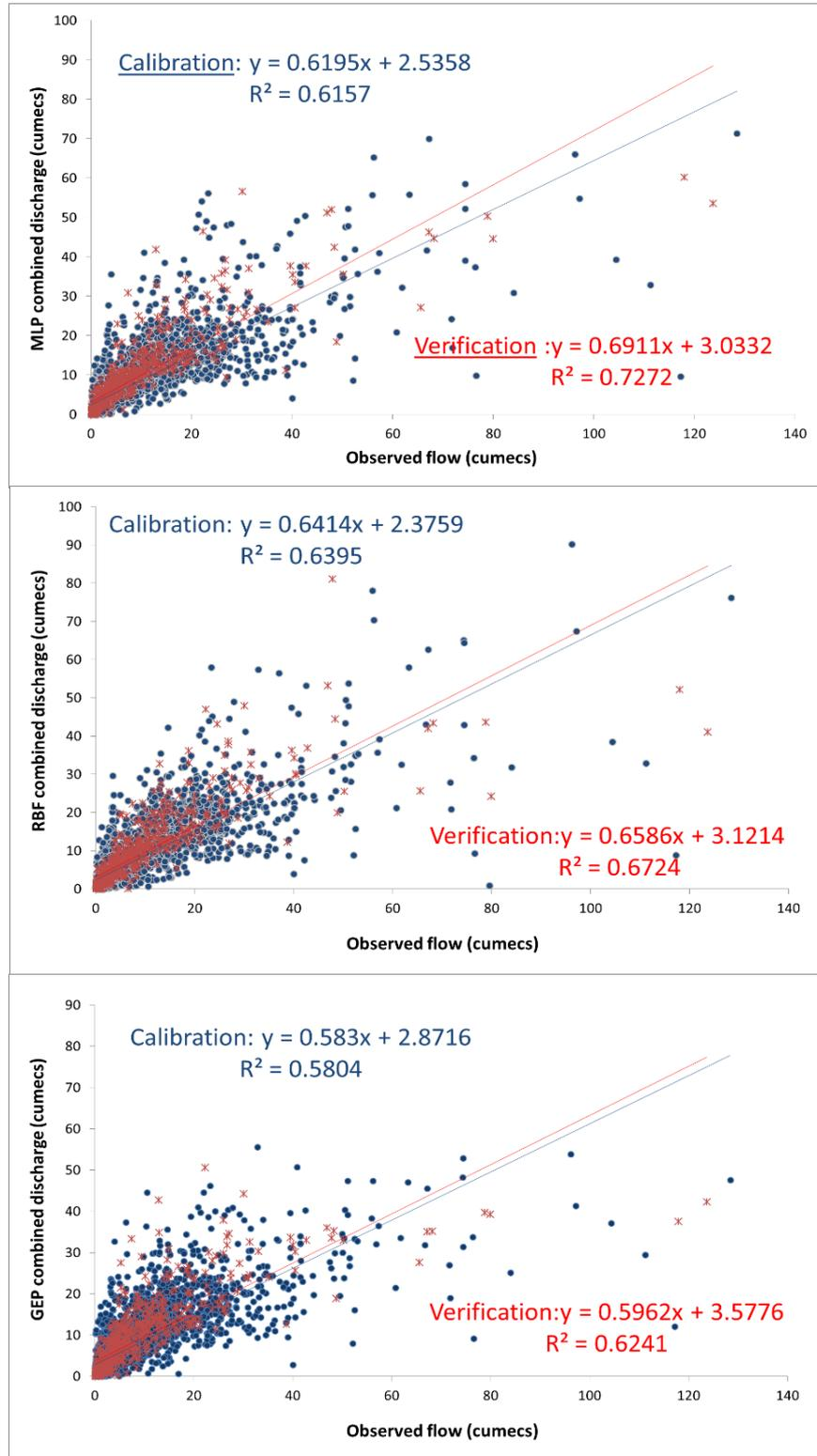
Figure 5.8: Scatter plots of observed discharge versus three combined models (i.e. RBF, MLP and GEP) at Mae Tuen River catchment during the time series, 4/01/1991 to 31/12/2002
