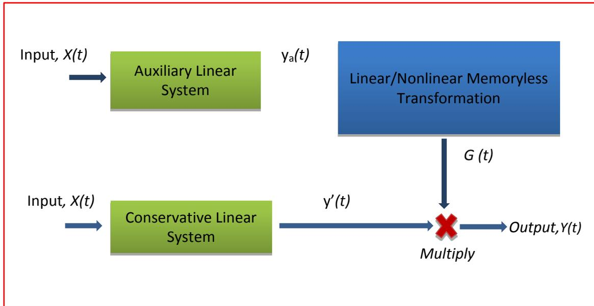
Figure 4.2: Schematic diagram of the Linearly Varying Gain Factor Model (Ahsan and O'Connor, 1994)
