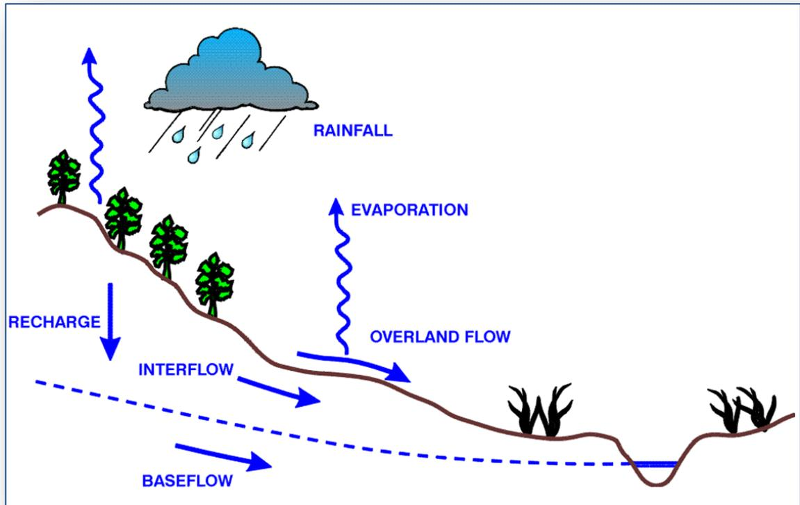
Figure 4.1: Schematic diagram of rainfall-runoff process
