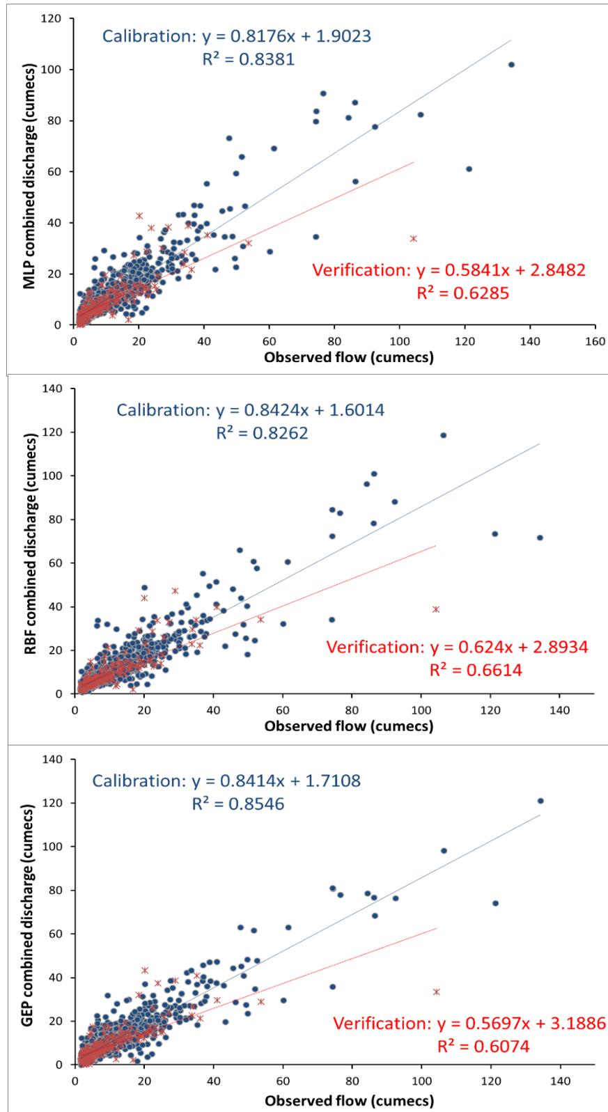
Figure 5.9: Scatter plots of observed discharge versus three combined models (i.e. RBF, MLP and GEP) at Ohinemuri River catchment during the time series, 1/01/1990 to
