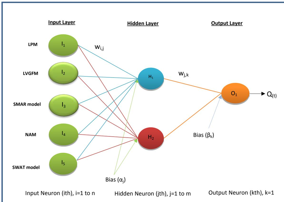
Figure 5.1: Network diagram showing the connection weights of MLPNN structure
