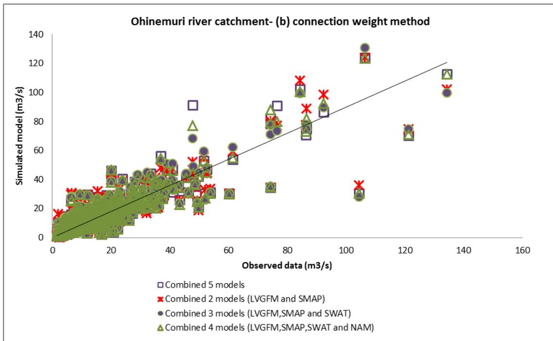
Figure 6.2: Scatter plot of simulated discharge between two variables for Ohinemuri River catchment: (a) Garson's algorithm and (b) Connection weight approach
