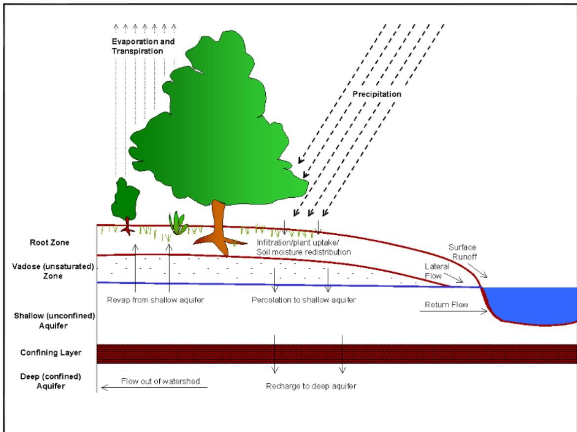
Figure 4.5: Schematic of the SWAT model representation of the hydrological process (Neitsch et al. 2009)
