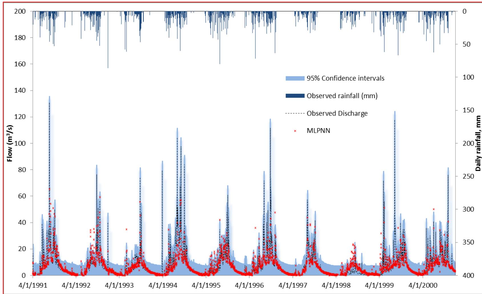
Figure 7.3: The 95% confidence intervals of the trained MLPNN combination system for the Mae Tuen River catchment
