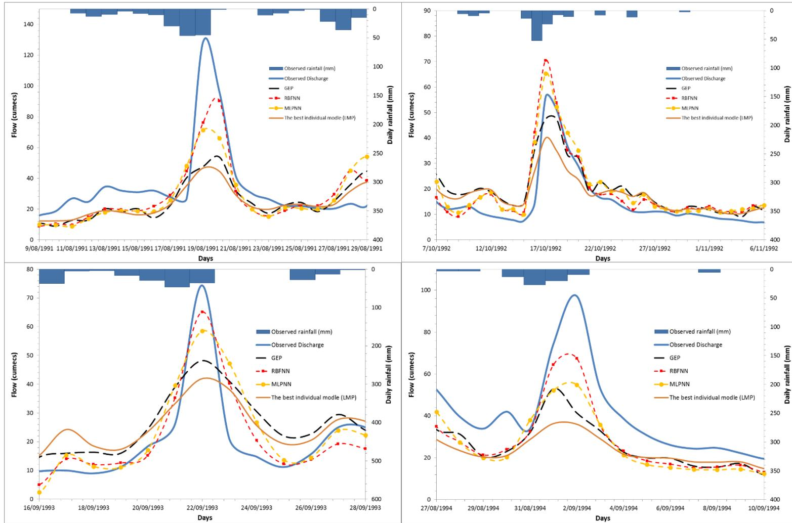
Figure 5.6: Comparison of the observed and simulated flood hydrographs of combined model of Mae Tuen River catchment
