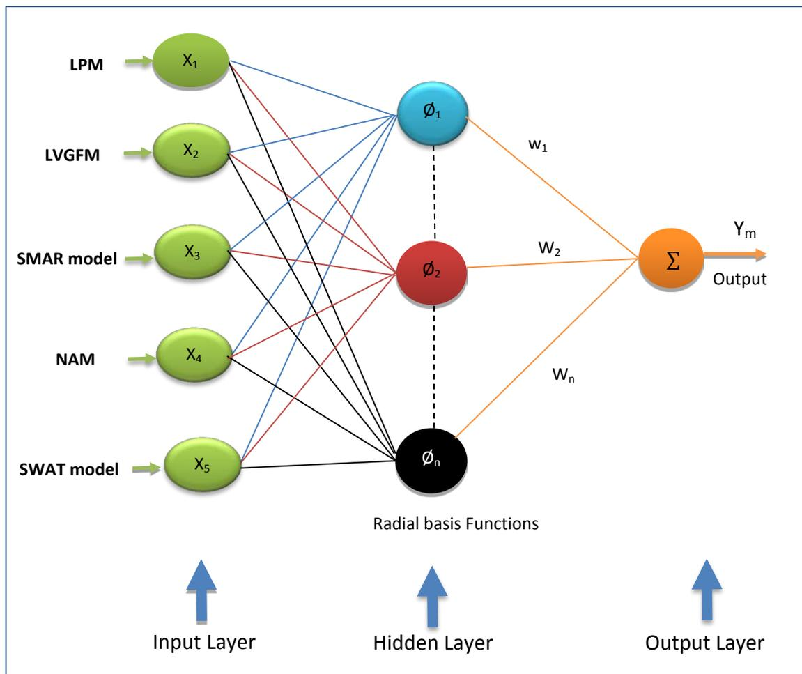
Figure 5.2: Network diagram showing the architecture of the radial basis function neural network
