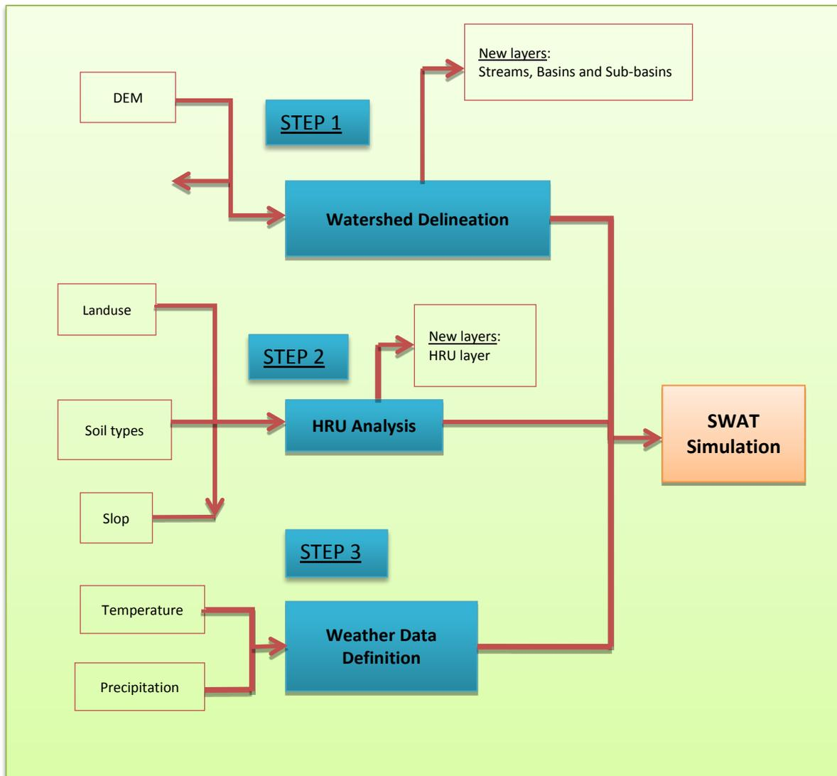
Figure 5.4: Schematic of SWAT model simulation
