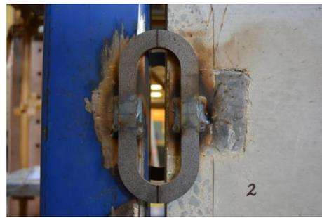
(b) Typical O-connector condition post-test (PreWEC-FV-A)
