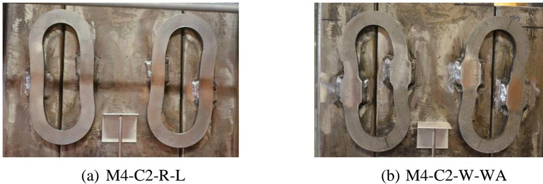
**Figure 3.7 – Typical O-connector deformed shape during tests**
