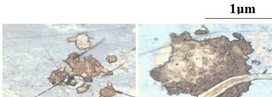
Figure 4.37. Microscopy images of the visual appearance of poly-2-ABA grown on a Pt electrode surfaces.
