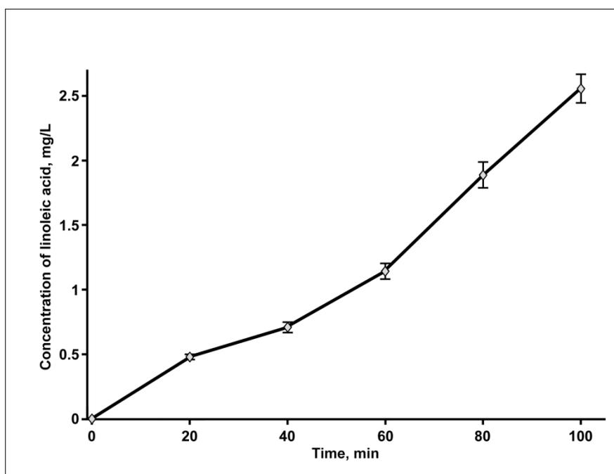
**Figure 5.2.** Liberation of linoleic acid from its substrate trilinolein by lipase under optimum conditions ( $40^\circ\text{C}$ ,  $\text{pH } 7.4$ ). The average concentration of corresponding compounds of three replicates per conditions displayed
