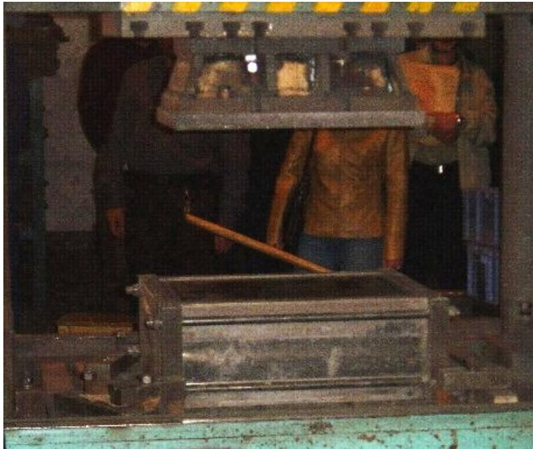
Figure 2-1: “Green” brick during pressing in the mold box (Courtesy LIRR).
