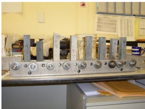
*Figure 6-2: Samples mounted in the metal frame before insertion in the reduction cell. Sample B, second from the left, was fractured during shipping and thus shorter than the remaining samples in the trial.*
