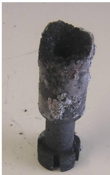
*Figure 5-10: Corroded sparging head.*
