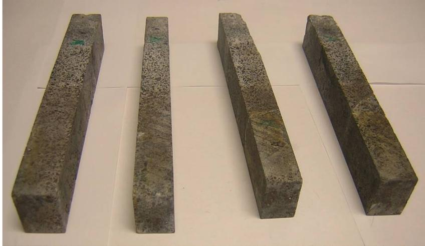
Figure 6-53: SNBSC sample after soaking treatment for 48 hours. No damage observed on the samples except colour change.
