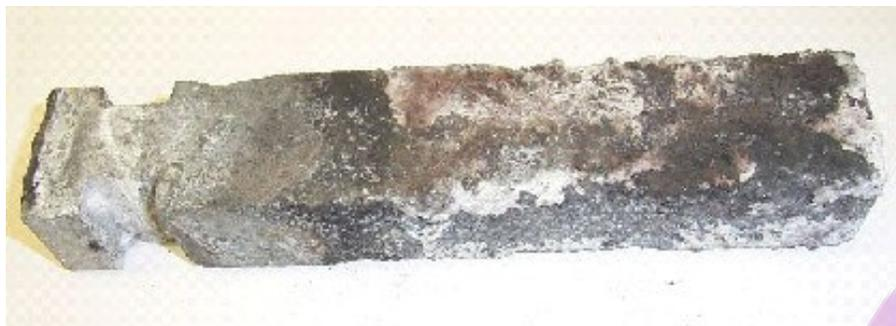
*Figure 6-5: Sample D2 removed after 30 hours partially immersion in the cell.*
