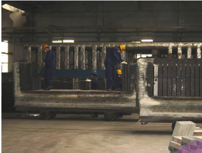
Figure 2-2: SNBSC bricks are stacked onto trolleys before nitridation (Courtesy LIRR).
