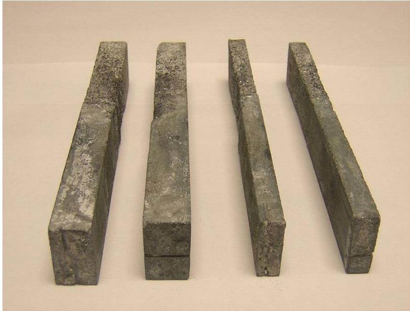
Figure 6-30: Four samples cut from brick H that were tested in the same experiment. On the right thinner samples that showed higher correlation between corrosion rate and porosity level compared to the wider samples (on the left).
