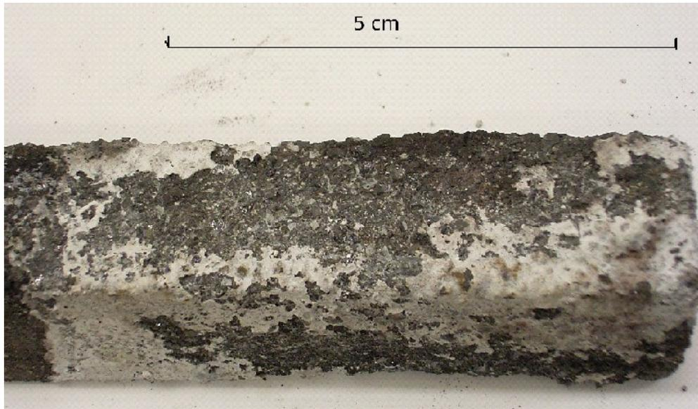
*Figure 3-18: SNBSC sample taken out of industrial scale cell after 30 hours of immersion half dipped in the bath [This work].*
