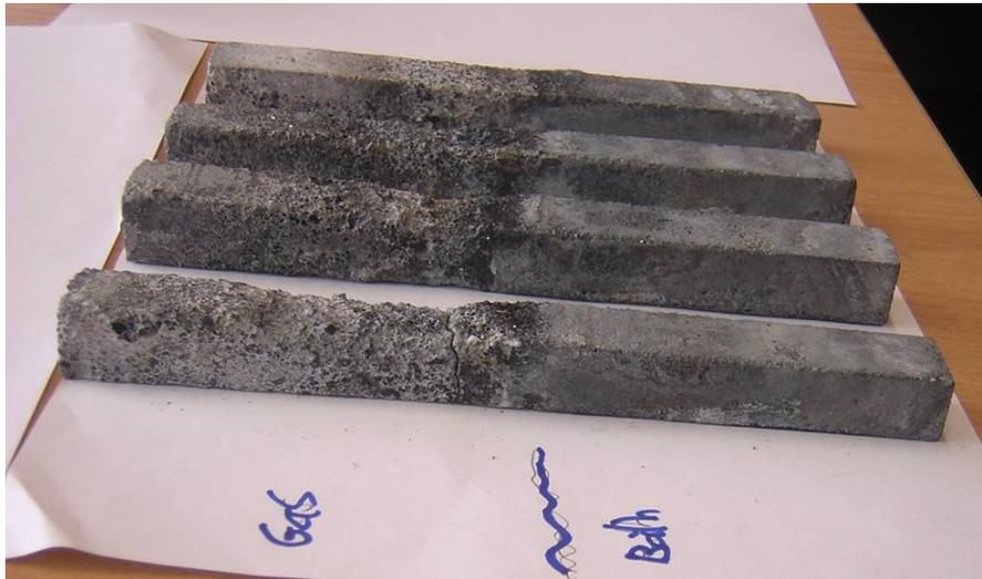
*Figure 6-52: SNBSC samples (25x20x185mm) after corrosion test. Degradation of the samples is observed mainly in the bath-gas interface and in gas phase.*
