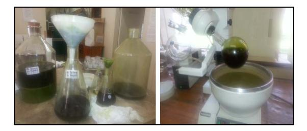
Figure 5.4: Crude extract acetone-bulk extraction processes (left) and drying process with a rotary evaporator (right)
