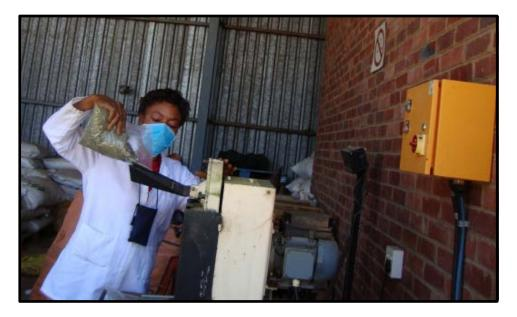
Figure 5.3: Grinding processes of dried leaves of *Searsia undulata* using a Macsalab Mill
