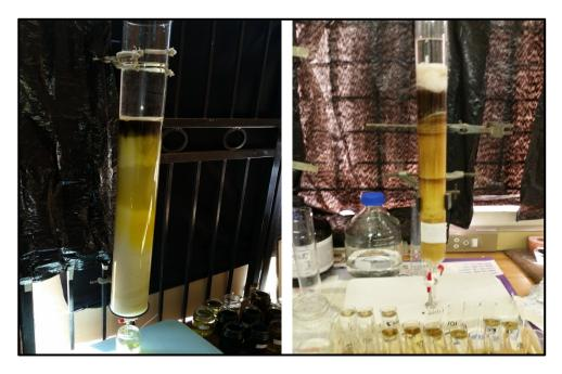
Figure 5.5: Column chromatography used for fractionation
