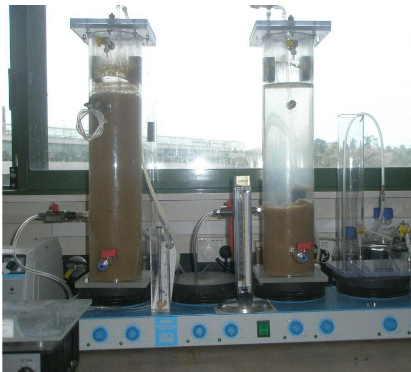
Figure 6.4 Bioreactors for 3 litres of denitrifying cultures
