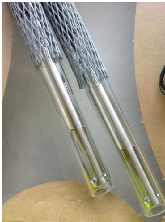
Figure 6.6. Unisense Clark type N 2 O microsensors
