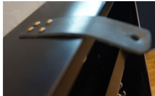
Figure 66 - Showing the leather strap mounted with rivets
