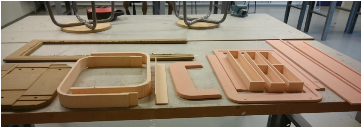
Figure 31- Showing the components that have been milled
