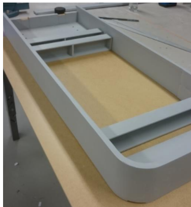
Figure 38 - Showing the frame and shelves covered in several layers of filler
